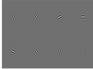
**Fig. 2.** An example of Gabor filters with a large frequency and different orientations
