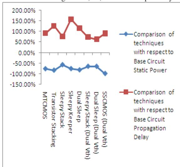
Fig. 14. Simulation Results of CMOS Inverter at 180nm
