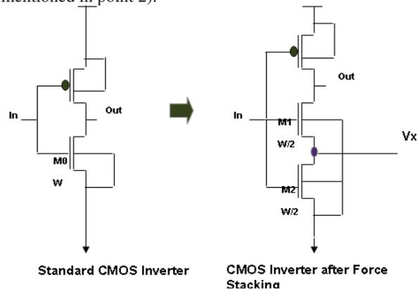
Fig. 5. Transistor Stacking
