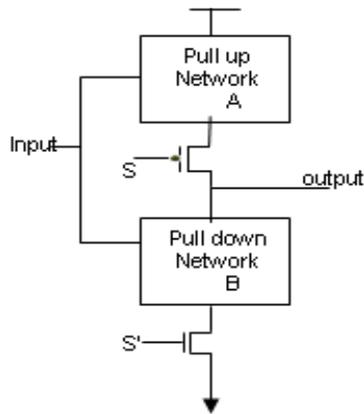
Fig. 4. Transistor Gating Technique
