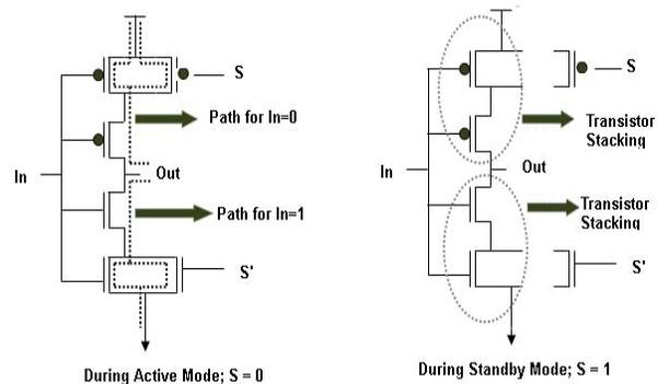
Fig. 8. Working of Sleepy stack
