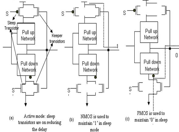
Fig. 9. Working of Sleepy Keeper
