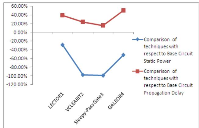
Fig. 17. Simulation Results of 2 Input NAND gate
