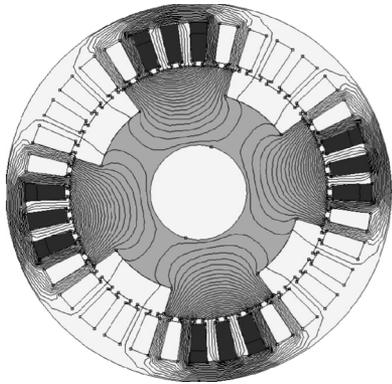
Fig. 12. Flux distribution in q-axis.
