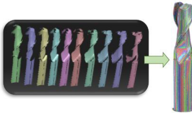
Fig. 5. Different perspectives of the analyzed object (left) and the result of the alignment (right)
