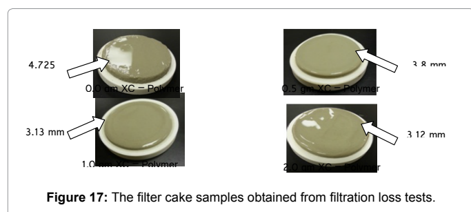
Figure 16: Effect the concentration of XC-Polymer on the thickness of filter cake.
