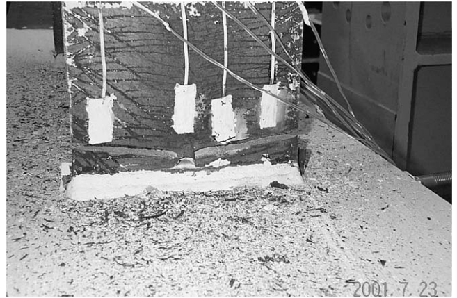
Fig. 15. Brittle fracture of beam top flange (specimen PN600-SB).
