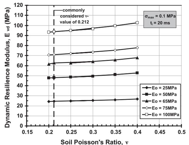
Figure 8 Influence of the soil Poisson's ratio on the  $E_{vd}$  modulus.
