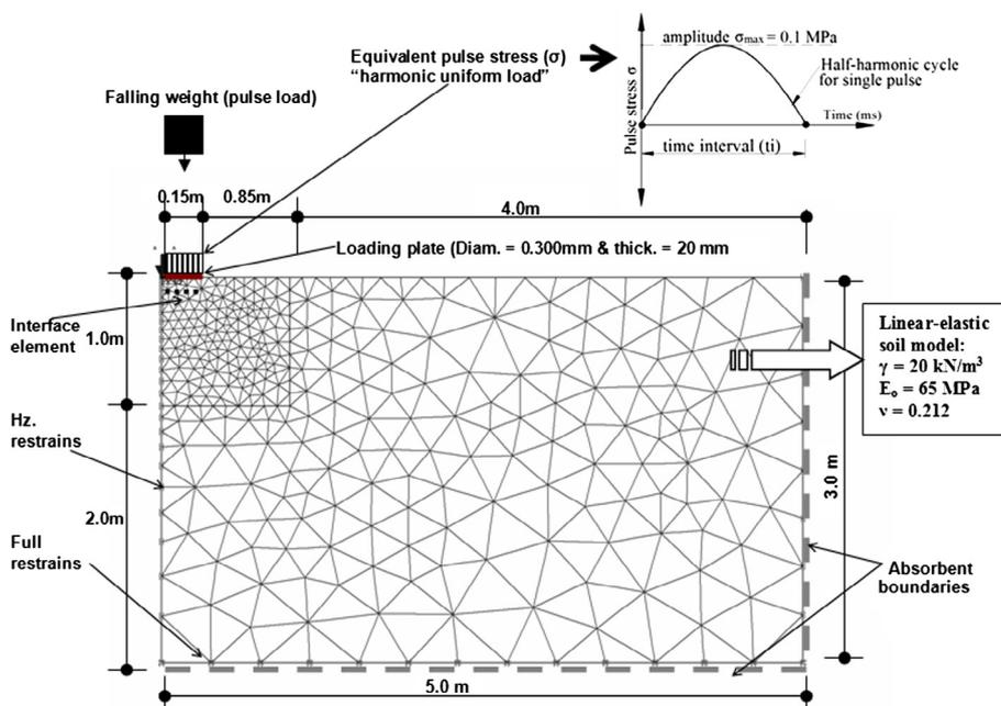
Figure 3 Geometry, boundary conditions and generated mesh of the finite element model.
