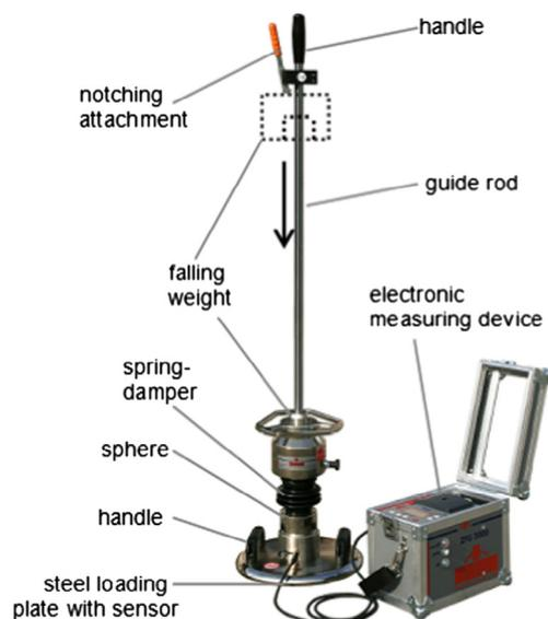
Figure 1 Details and components of the German LFWD.
