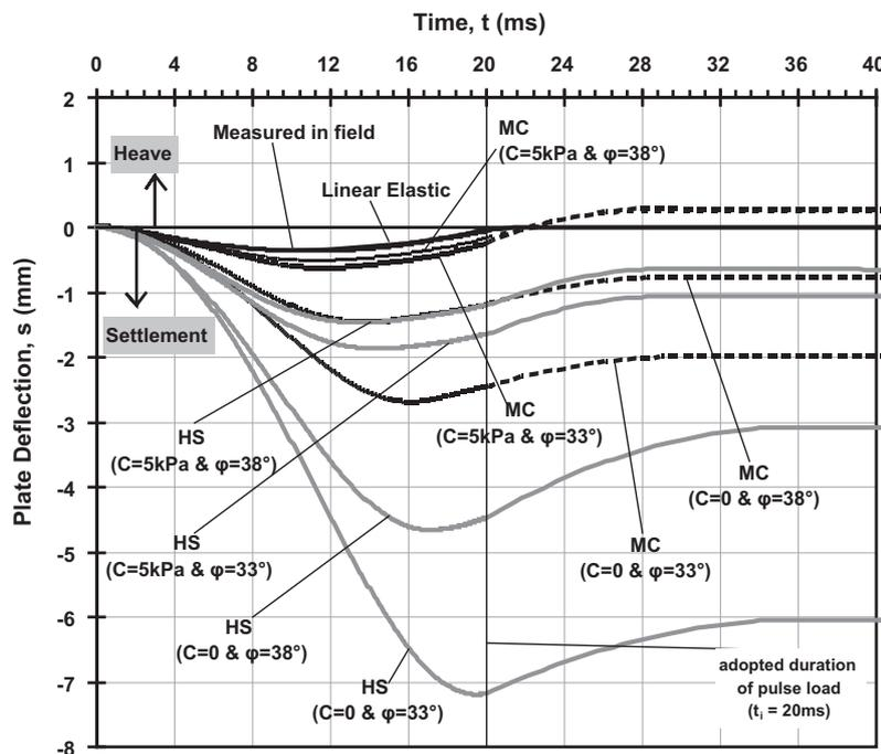
Figure 7 Calculated plate deflection from different soil models due to a single pulse.
