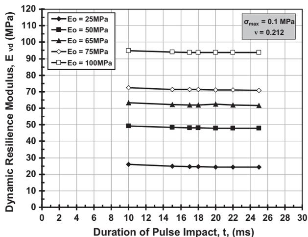
**Figure 9** Influence of the duration (time) of pulse impact on the  $E_{vd}$  modulus.
