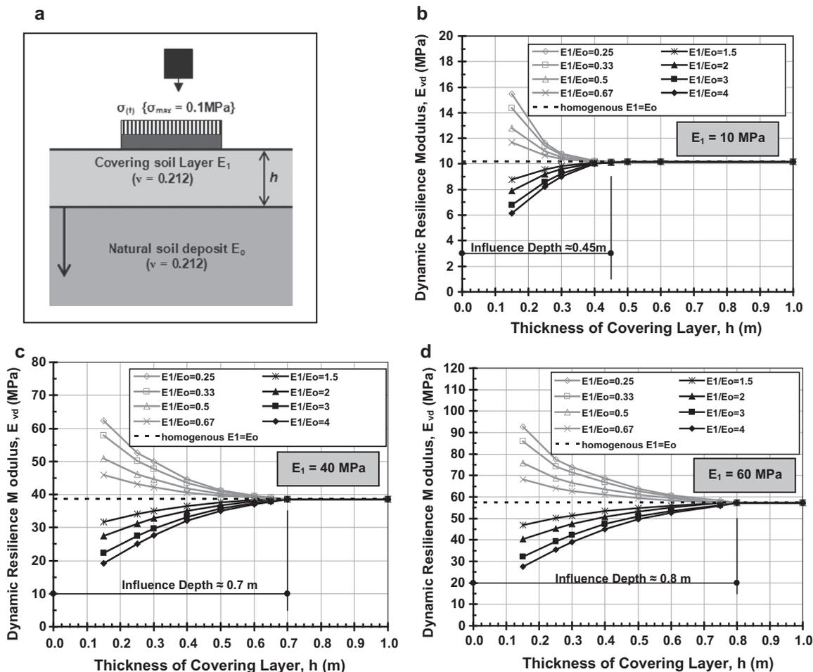
**Figure 10** Influence of soil stratification on the  $E_{vd}$  modulus: (a) proposed layered soil system, (b) case of  $E_1 = 10$  MPa, (c) case of  $E_1 = 40$  MPa, and (d) case of  $E_1 = 60$  MPa.
