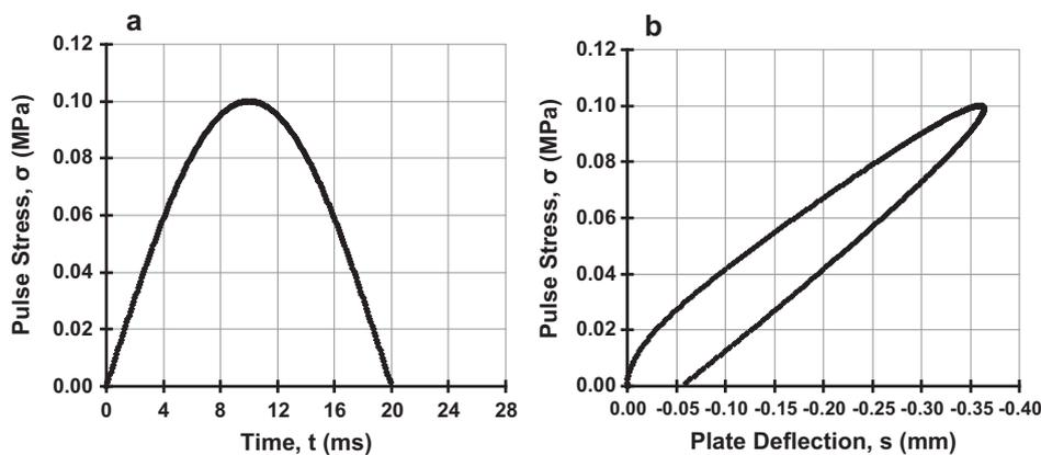
Figure 6 Curves from the finite element calculations: (a) development curve of pulse stress, and (b) development curve of plate deflection (stress loop).
