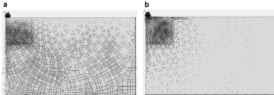
**Figure 5** Samples of results from the finite element model: (a) principal stresses field, and (b) principal total strains field.
