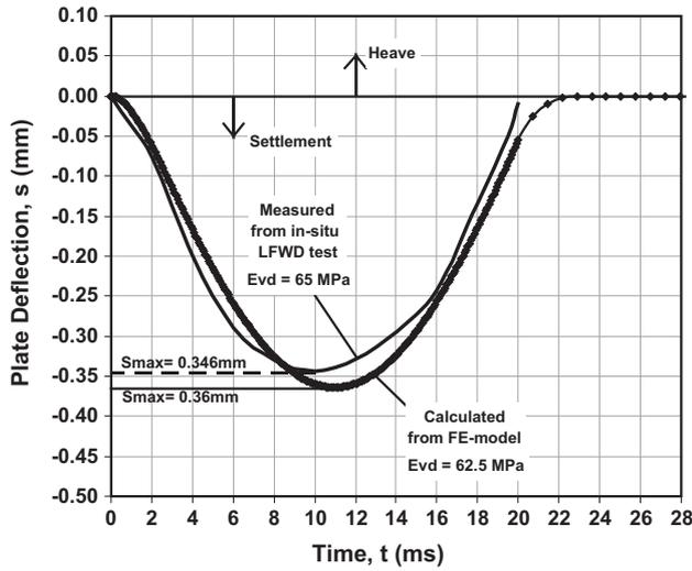
**Figure 4** Measured and calculated plate deflection during a single pulse of LFWD.
