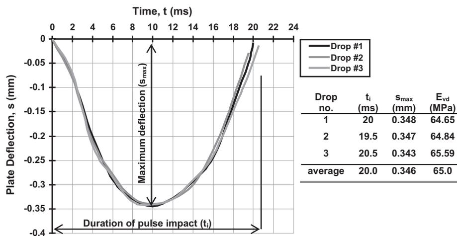
Figure 2 Field records of the implicated LFWD test.
