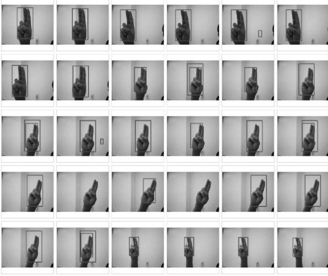
Fig.9. Some detection results for the “two-finger” posture with the trained cascade classifier.
