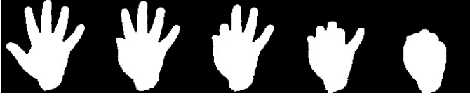
Fig. 3. Some transient, false gestures are detected during the process of the gesture changing from ‘palm’ to ‘fist’.
