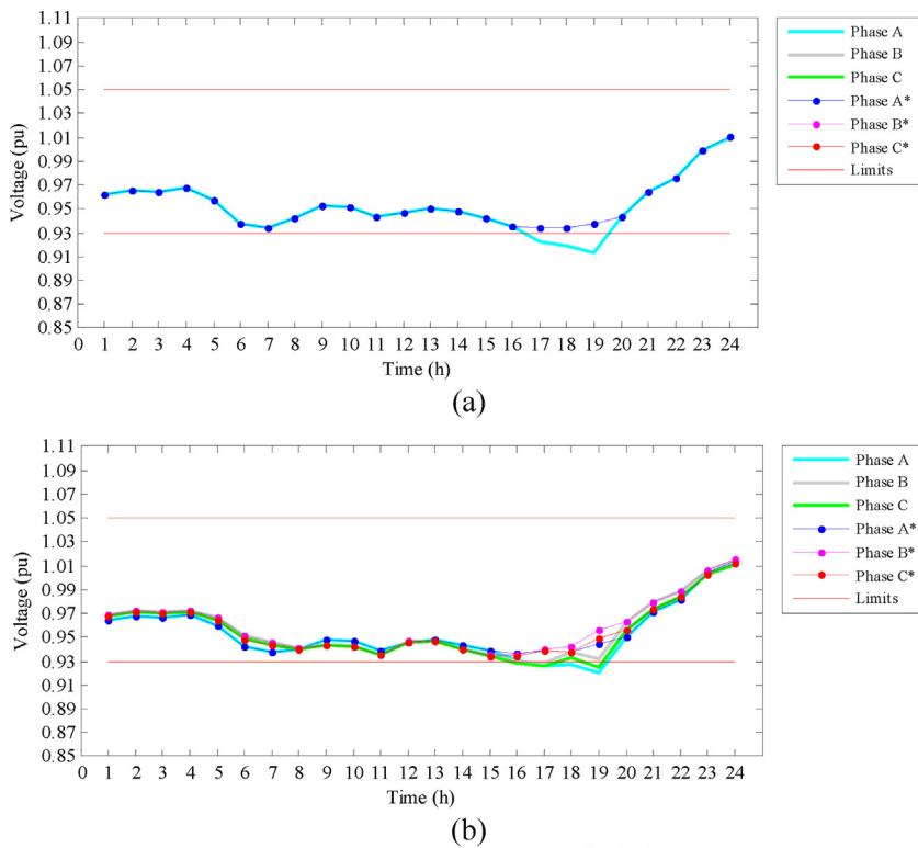
**Fig. 11.** Voltage profile before (phases ABC) and after (phases A\*B\*C\*) the coordinated VVC application in (a) Bus 12 and in (b) Bus 29.
