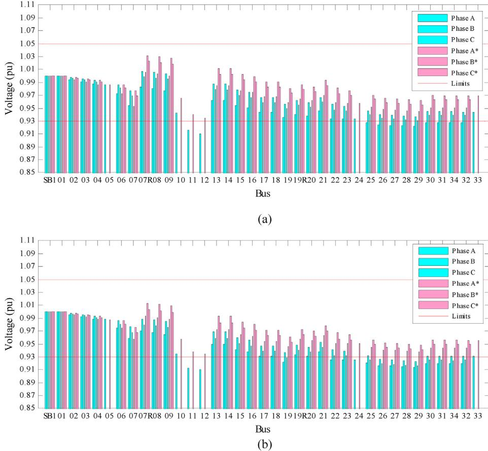
**Fig. 10.** Voltage behaviors to the maximum demanding time (19 h) before (phases ABC) and after (phases A\*B\*C\*) the coordinated VVC application (a) with CM disabled and (b) with CM and EM enabled.
