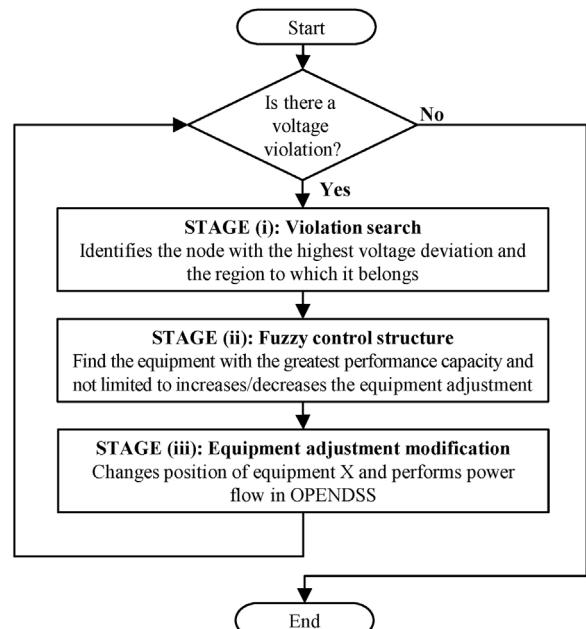
**Fig. 3.** Main stages of the coordinated VVC algorithm.
