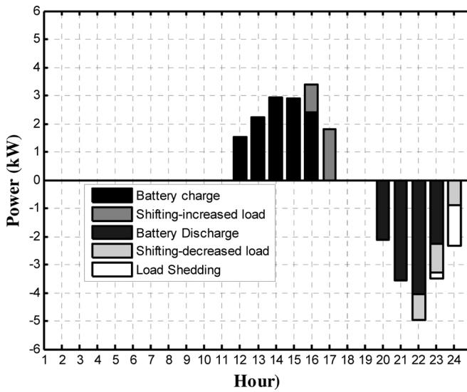
Fig. 7. Control actions performed in phase 1.
