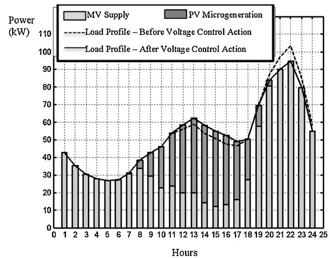
Fig. 9. Balance of power before/after voltage control action.
