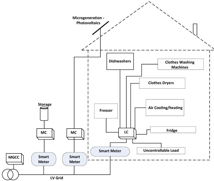
**Fig. 1.** Proposed control LV architecture for residential customers.
