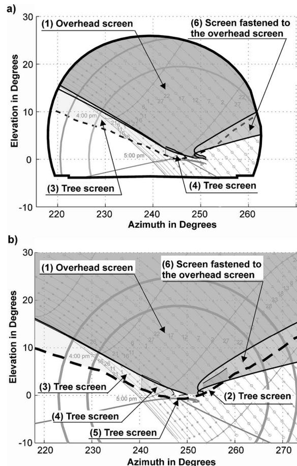
Fig. 11. Glare protection measures (a) inside the tunnel; (b) at the daylight adaptation point
