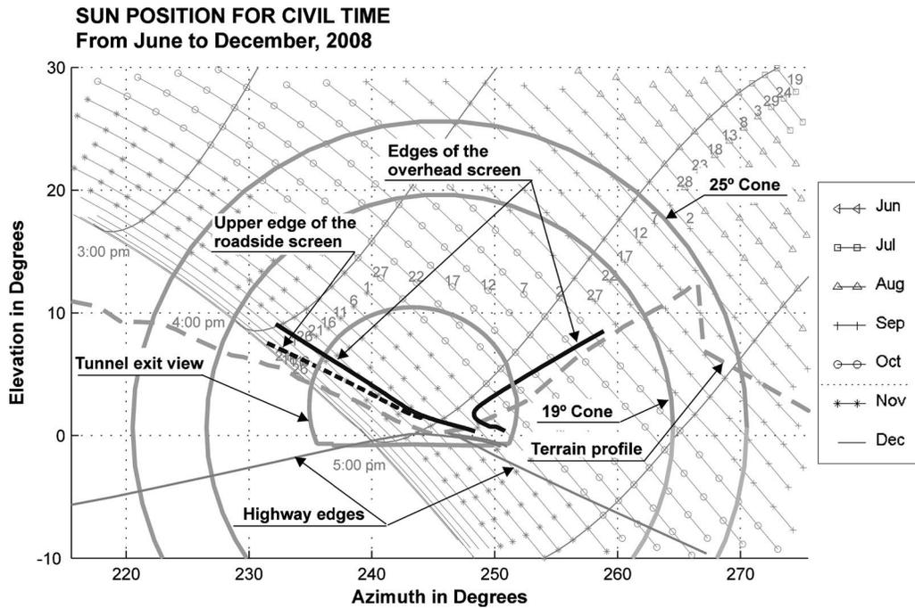
**Fig. 7.** Cylindrical chart with all the variables involved in local glare countermeasure effectiveness analysis
