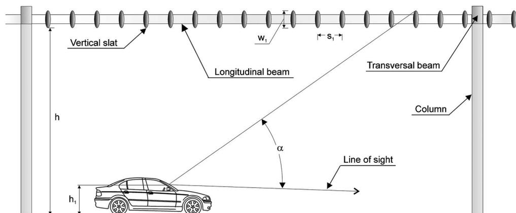
Fig. 5. Example of discontinuous overhead screen design on level terrain
