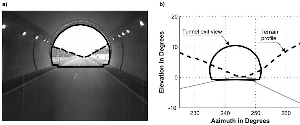
Fig. 2. Problem factors: terrain profile and tunnel exit view (a) reality; (b) representation in a cylindrical chart
