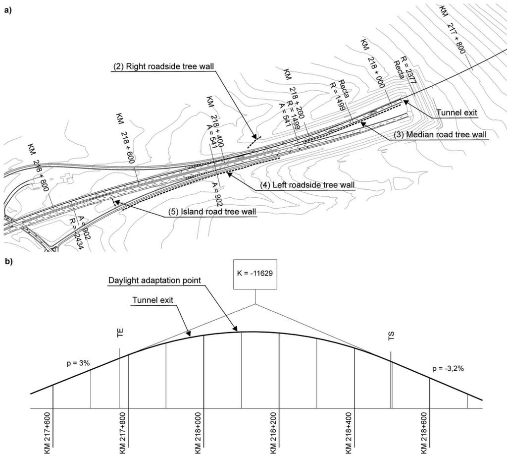
Fig. 10. (a) Road plan showing location of sun glare countermeasures layout; (b) road profile
