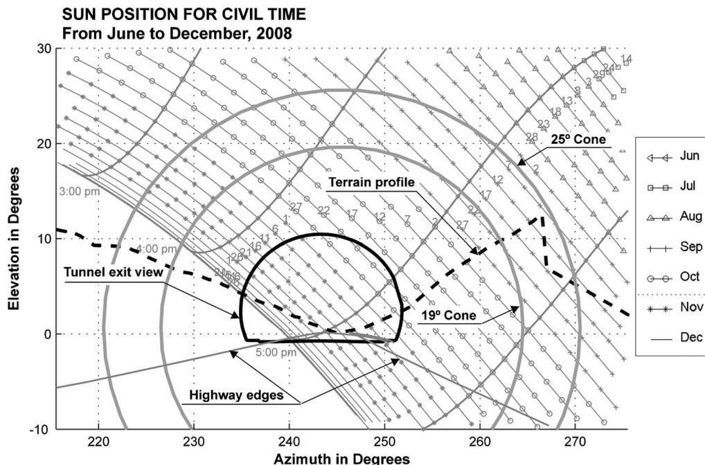
Fig. 3. Local glare analysis at km 217+920 National Motorway A-5 (Spain)
