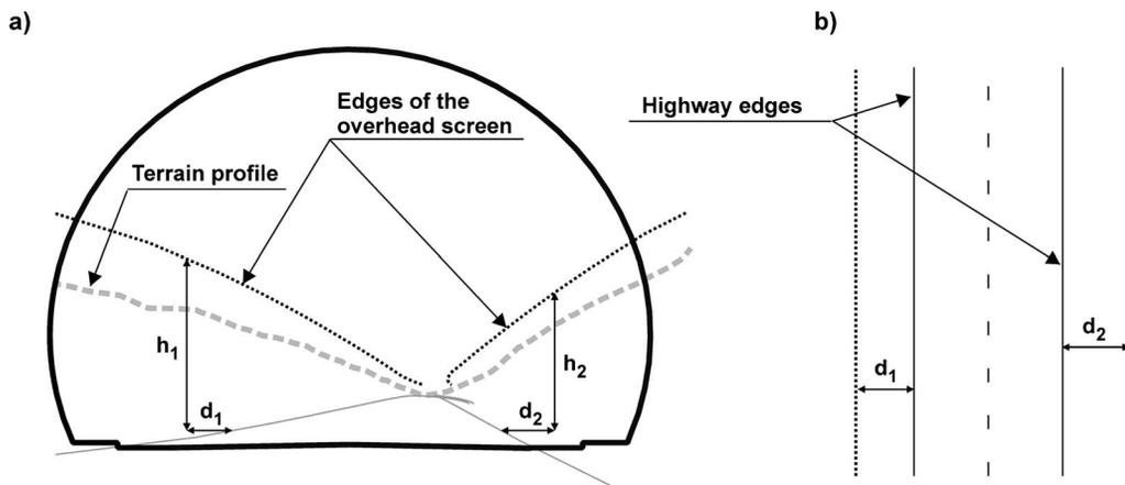
Fig. 6. Geometric definition of an overhead screen (a) perspective; (b) plan
