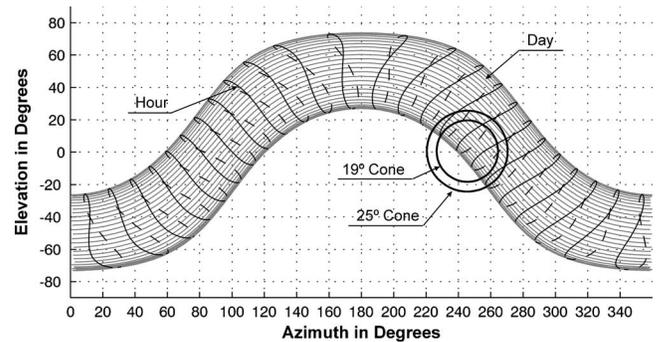
Fig. 1. Sun path and glare cones at km 217+920 National Motorway A-5 (Spain)
