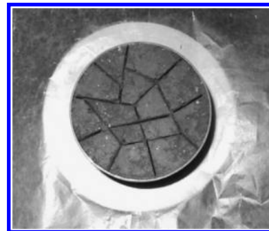
Figure 2. Artificially cracked sample No. 1 with 3.2% crack volume. (The crack volume for sample No. 2 was 4.4%).
