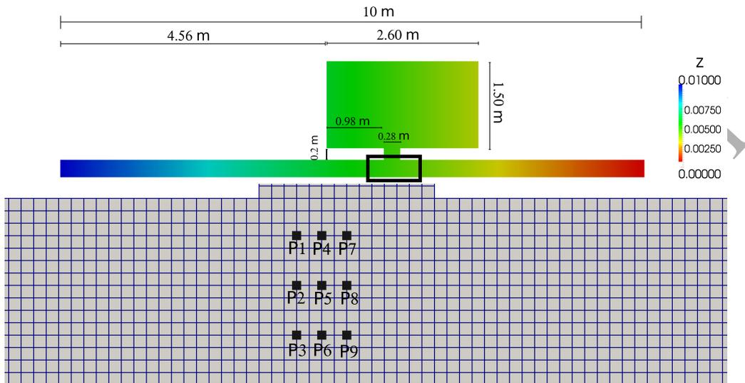
Figure 5: Laboratory test case. Full set-up (upper) and detail of the squared mesh and the location of the probes (lower)
