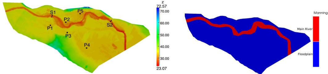
Figure 13: Ponzano reach: Topography and location of section and probes (left) and Manning roughness map (right)
