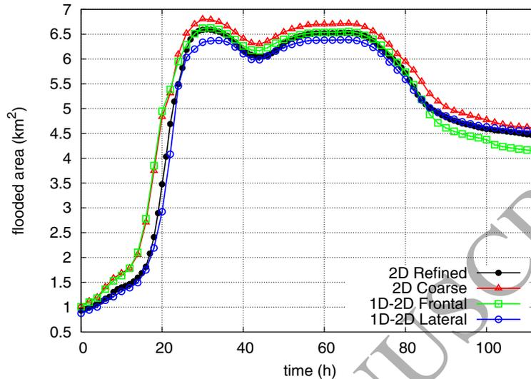
Figure 19: Ponzano reach. Time evolution of the flooded area computed by each model
