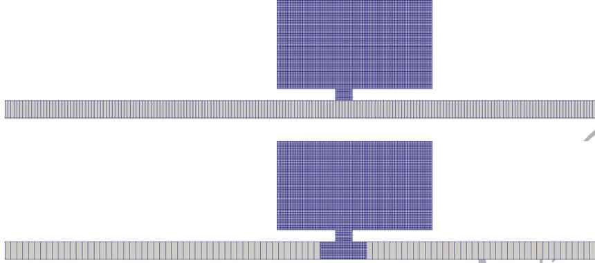
Figure 6: Laboratory test case: 1D-2D lateral (upper) and frontal (lower) configurations
