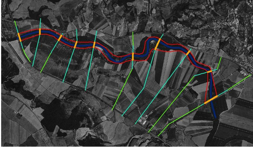
Figure 10: Aerial photograph of Ponzano area with original and interpolated 1D cross sections
