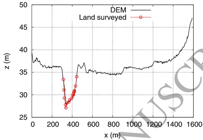
Figure 11: Comparison between the land surveyed and the DEM reconstructed extraction for section 5 in Ponzano reach
