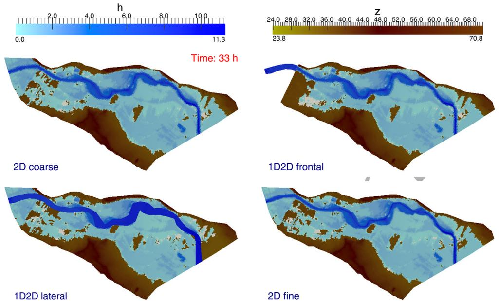
Figure 16: Ponzano reach: Flooded area at time  $t=33$  h. computed by the 2D coarse (upper left), 1D-2D frontal (upper right), 1D-2D lateral (lower left) and 2D fine model (lower right)
