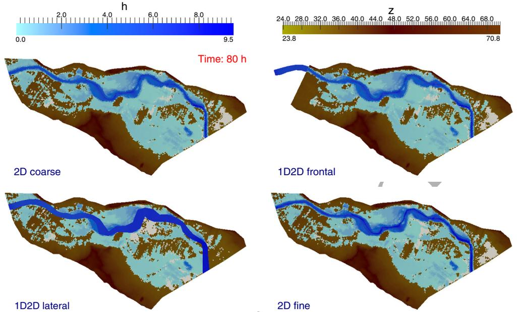
Figure 17: Ponzano reach: Flooded area at time  $t=80$  h. computed by the 2D coarse (upper left), 1D-2D frontal (upper right), 1D-2D lateral (lower left) and 2D fine model (lower right)
