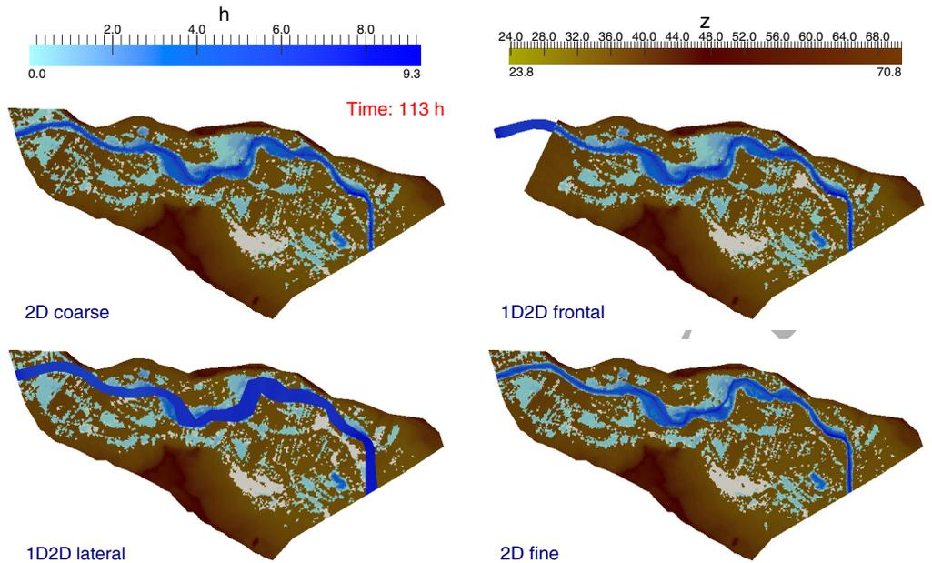
Figure 18: Ponzano reach: Flooded area at time  $t=113$  h. computed by the 2D coarse (upper left), 1D-2D frontal (upper right), 1D-2D lateral (lower left) and 2D fine model (lower right)
