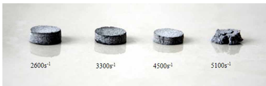
4 The macro-picture of the specimens after test under different strain rates. a At the strain rate of 2600 \text{s}^{-1} ; b at the strain rate of 3300 \text{s}^{-1} ; c at the strain rate of 4500 \text{s}^{-1}
