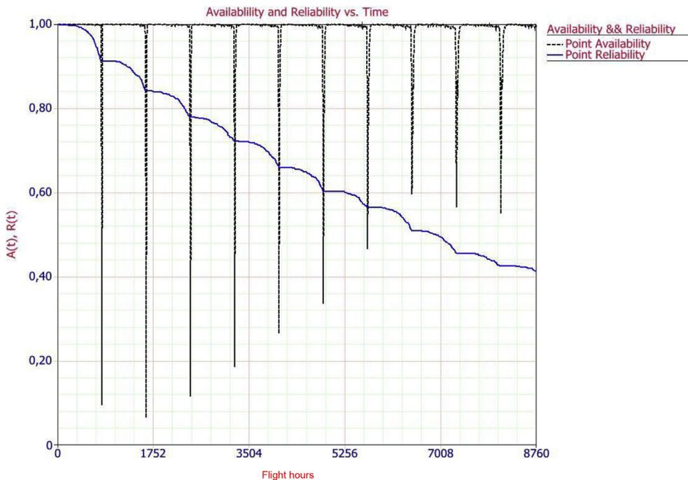
Fig. 12. Availability and reliability (two spare parts for A and E and one spare part for the others).
