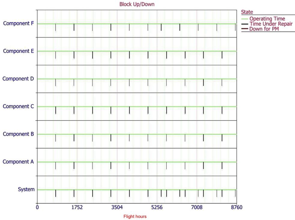
Fig. 11. Up/down patterns (two spare parts for A and E and one spare part for the others).
