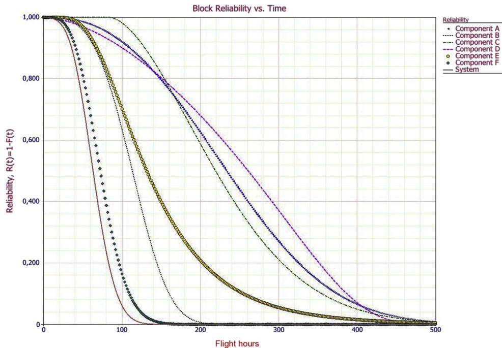
Fig. 3. Block reliability  $R(t)$  vs. flight hours.
