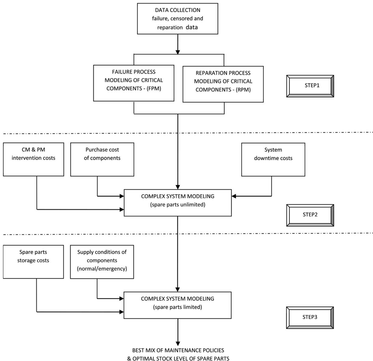
Fig. 1. Proposed method for the determination of the maintenance policy and the best inventory management strategy.
