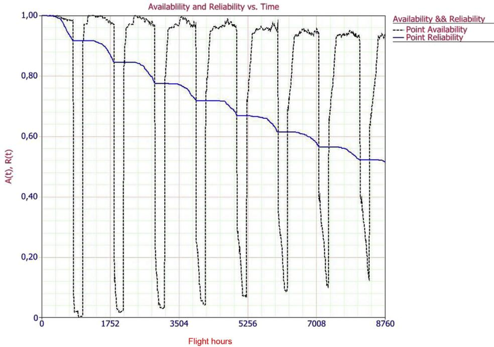
Fig. 7. System availability and reliability (no spare parts in stock).
