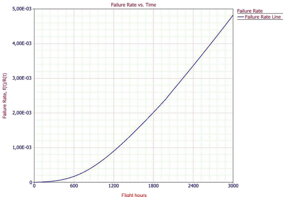
**Fig. 4.** System failure rate  $\lambda(t)$  vs. flight hours.
