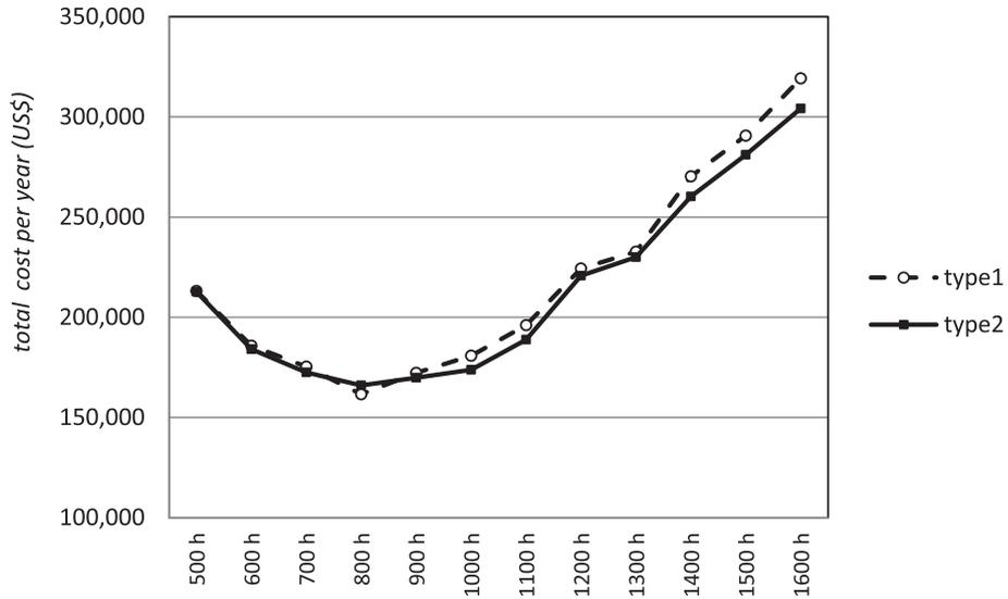
Fig. 5. Average value of total maintenance cost (Type 1 and Type 2 methods).
