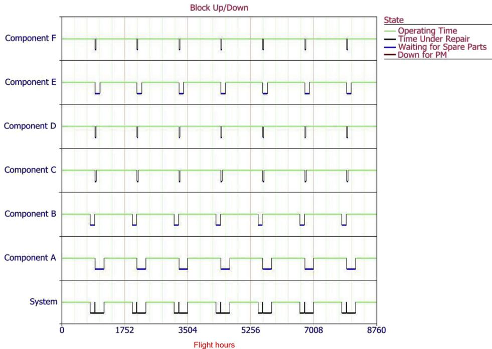
Fig. 6. Up/down patterns (no spare parts in stock).
