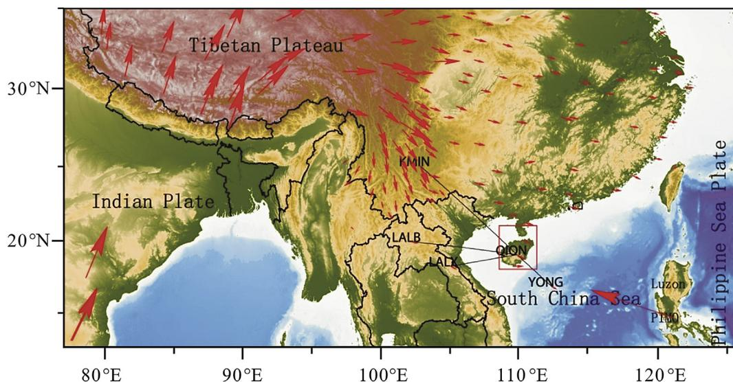
**Fig. 1 – GPS velocities relative to Eurasia in the period from 1999 to 2013. The red small box in the inset map shows the study region. Black lines between the two stations are the baselines in Table 1.**
