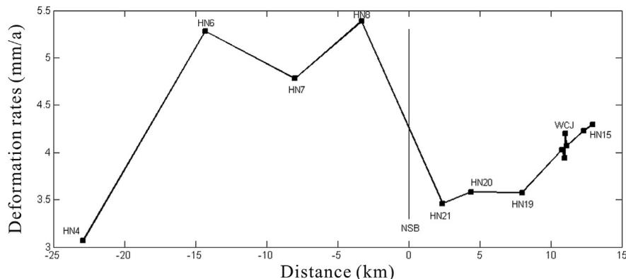
**Fig. 7 – Vertical deformation rates detected by precise leveling across the NSB. The solid line is the presumed fault. The distances are between the benchmarks and the center of the NSB.**
