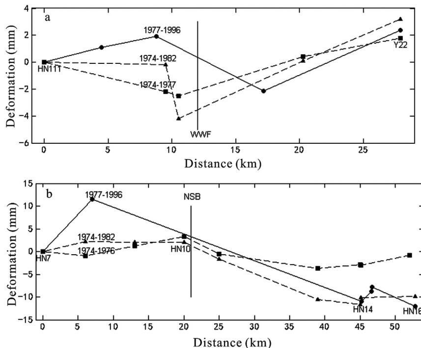
Fig. 6 – a) Vertical deformation from south to north for three periods. The deformation during 1974–1982 and 1974–1977 is from reference [13]. b) Vertical deformation from the west to east for three periods. The deformation during 1974–1982 and 1974–1976 is from reference [13].
