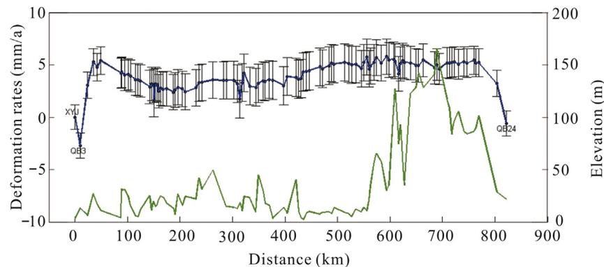
**Fig. 4 – Vertical deformation rates with error bars detected by precise leveling in the period from 1970s to 1990s (Blue line). The green line is the elevations.**
