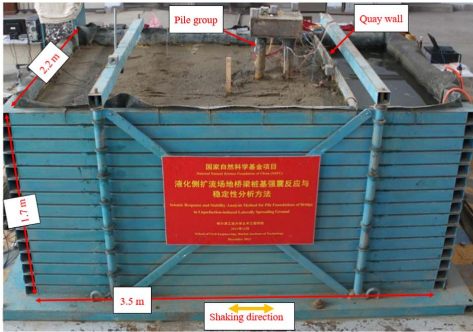
Fig. 1. Shake-table test on pile group.
