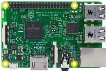
FIG. 5. Raspberry-Pi Hardware Platform
