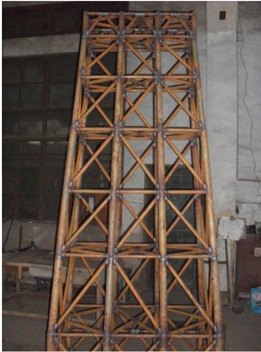
Fig. 5. The corrosion model of jacket.
