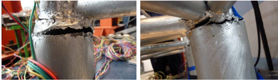
Fig. 13. Crack tearing deformation of the corrosion model.
