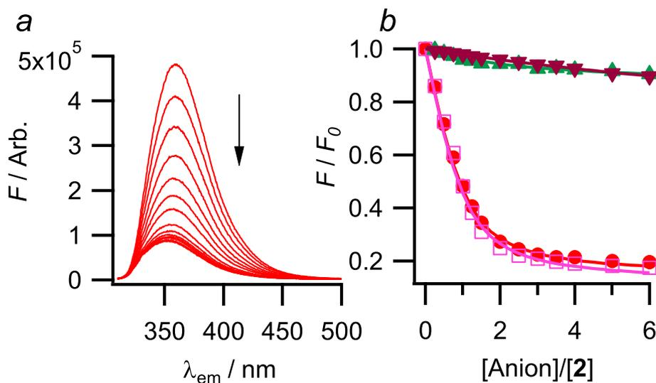
**Fig. 2.** (a) Fluorescence spectral titration of **2** with  $\text{AcO}^-$  in MeCN. (b) Fluorescence intensity changes of **2** at 358 nm upon the addition of anions in MeCN.  $\text{AcO}^-$  (●),  $\text{H}_2\text{PO}_4^-$  (□),  $\text{Cl}^-$  (▲), and  $\text{Br}^-$  (▼).  $[\mathbf{2}] = 1.0 \times 10^{-5} \text{ mol dm}^{-3}$ ,  $\lambda_{\text{ex}} = 301 \text{ nm}$  at 298 K.
