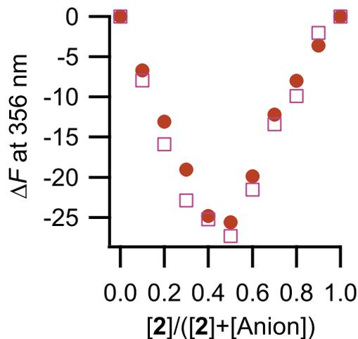
**Fig. 3.** Job plots of **2** with  $\text{AcO}^-$  (●) and  $\text{H}_2\text{PO}_4^-$  (□) in MeCN.  $[\mathbf{2}] + [\text{anion}] = 1.0 \times 10^{-5} \text{ mol dm}^{-3}$ .
