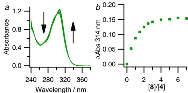
**Fig. 4.** (a) UV-vis spectral changes of **4** upon the addition of dibutylbarbituric acid (**8**) in  $\text{CHCl}_3$ . (b) Absorbance changes of **4** at 314 nm upon the addition of **8** in  $\text{CHCl}_3$ .  $[\mathbf{4}] = 2.0 \times 10^{-5} \text{ mol dm}^{-3}$  at 298 K.
