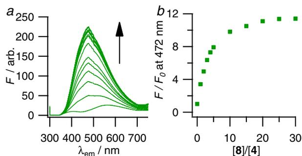
**Fig. 5.** (a) Fluorescence changes of **4** upon the addition of **8** in  $\text{CHCl}_3$ . (b) Fluorescence spectral changes of **4** at 472 nm upon the addition of **8** in  $\text{CHCl}_3$ .  $[\mathbf{4}] = 5.0 \times 10^{-6} \text{ mol dm}^{-3}$ ,  $\lambda_{\text{ex}} = 298 \text{ nm}$  at 298 K.
