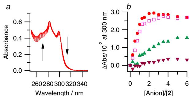
Fig. 1. (a) UV-vis spectral titration of **2** with AcO<sup>−</sup> in MeCN. (b) Absorbance change of **2** at 280 nm upon the addition of various anions in MeCN. AcO<sup>−</sup> (●), H<sub>2</sub>PO<sub>4</sub><sup>−</sup> (□), Cl<sup>−</sup> (▲), and Br<sup>−</sup> (▼). [2] = 2.0 × 10<sup>−5</sup> mol dm<sup>−3</sup> at 298 K.
