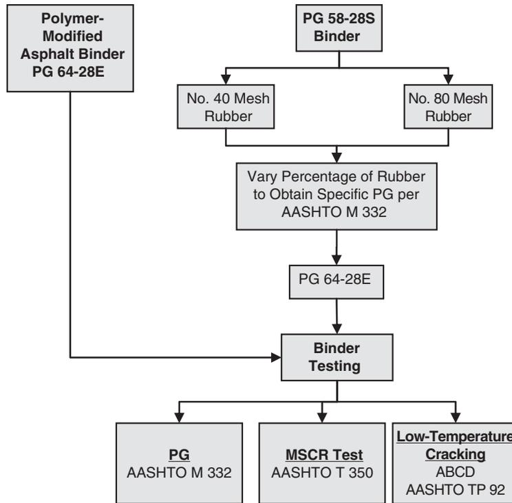
FIGURE 1 Experimental plan for binder (ABCD = asphalt binder cracking device).
