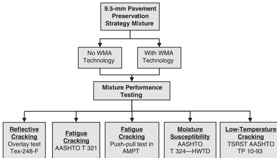
FIGURE 2 Experimental plan for mixture (AMPT = asphalt mixture performance tester; HWT D = Hamburg Wheel Tracking Device; TSRST = thermal stress restrained specimen test).
