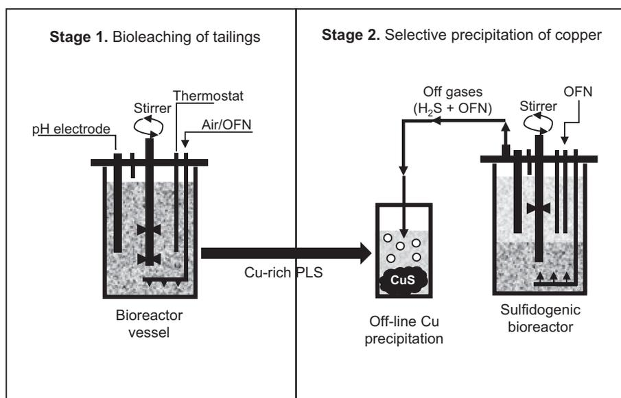
**Fig. 1.** Schematic representation (not in scale) of the reactors used during the bioleaching experiments (stage 1) and the offline precipitation of copper using a low pH sulfidogenic bioreactor (stage 2).
