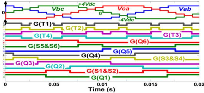
Fig. 2. Simulated waveforms of  $V_{ab}$ ,  $V_{bc}$ , and  $V_{ca}$  with corresponding switching gate signals for the proposed inverter at fundamental frequency  $f = 50$  Hz.
