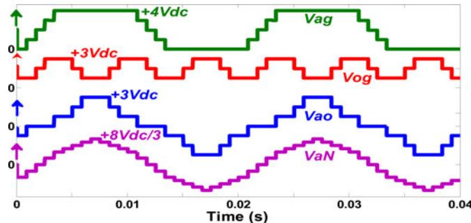
Fig. 3. Simulated waveforms of  $V_{ag}$ ,  $V_{og}$ ,  $V_{ao}$ , and  $V_{aN}$  for the proposed inverter  $f = 50$  Hz.
