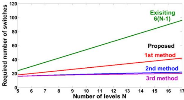
Fig. 8. Comparison of required number of switches among existing inverters and the proposed topology.
