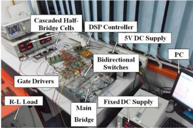
Fig. 11. Prototype of the proposed multilevel inverter.
