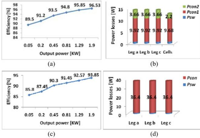
Fig. 9. Power loss and efficiency comparison. For the proposed inverter: (a) output power versus efficiency, (b)  $P_{con}$  and  $P_{sw}$  distribution among legs  $a$ ,  $b$ ,  $c$ , and CHB cells for  $M_a = 1$  and  $P_{out} = 1.287$  kW. For the NPC inverter: (c) output power versus efficiency and (d)  $P_{con}$  and  $P_{sw}$  distribution among legs  $a$ ,  $b$ , and  $c$  for  $M_a = 1$  and  $P_{out} = 1.285$  kW.
