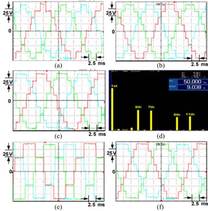
Fig. 14. (a) Three-line-to-line voltages at  $M_a = 0.9$ , (b) three-line-to-line voltages at  $M_a = 1.05$ , (c) three-line-to-line voltages at  $M_a = 1.15$ , (d) THD% at  $M_a = 1.15$ , (e) three-line-to-line voltages at  $M_a = 0.8$ , and (f) three-line-to-line voltages at  $M_a = 1.3$ .
