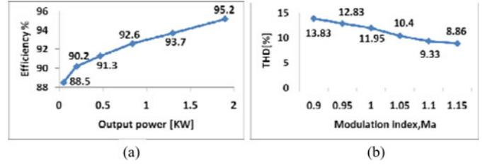
Fig. 15. Experimental results of (a) output power versus efficiency for the proposed inverter and (b) line-to-line voltage THD% versus  $M_a$  for  $V_{dc} = 75$  V.
