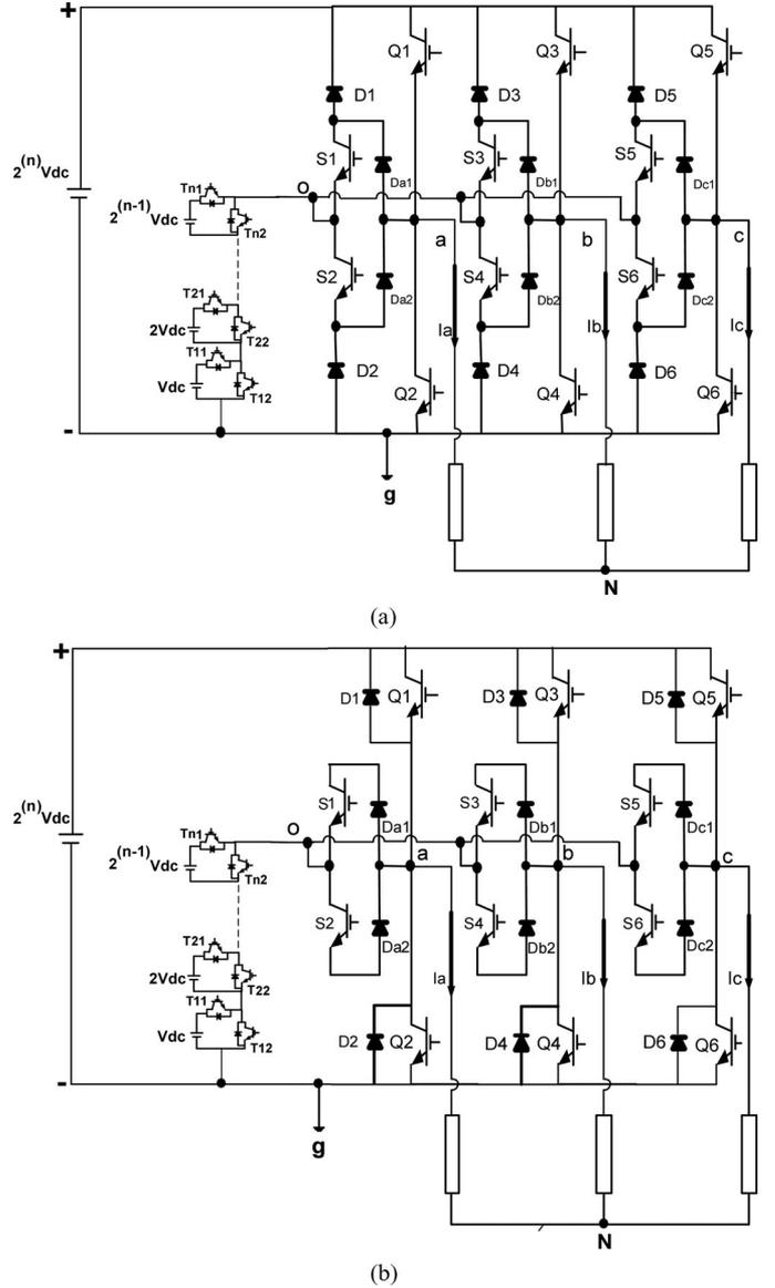
Fig. 7. Circuit diagram of the proposed three-phase  $N$ -level multilevel inverter (third method).
