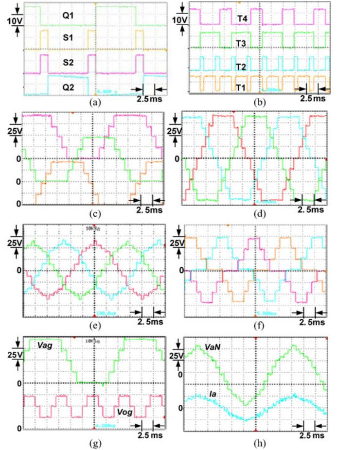
Fig. 13. (a) Switching gate signals of Q1, S1, S2, and Q2, (b) switching gate signals of T1, T2, T3, and T4, (c) three-line-to-ground voltages, (d) three-line-to-line voltages, (e) three-line to neutral voltages, (f) three-line to midpoint voltages, (g) midpoint to ground and line-to-ground voltages, and (h) load current  $I_a$  and line-to-neutral voltage  $V_{aN}$ .
