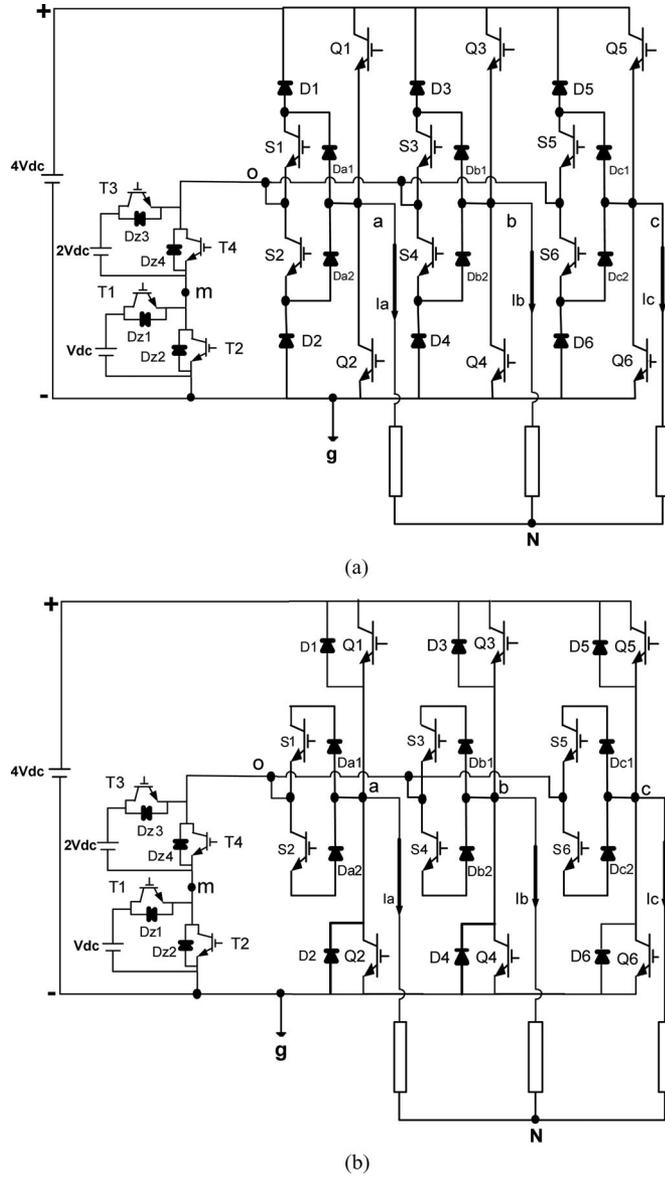
Fig. 1. Circuit diagram of the proposed three-phase five-level multilevel inverter.
