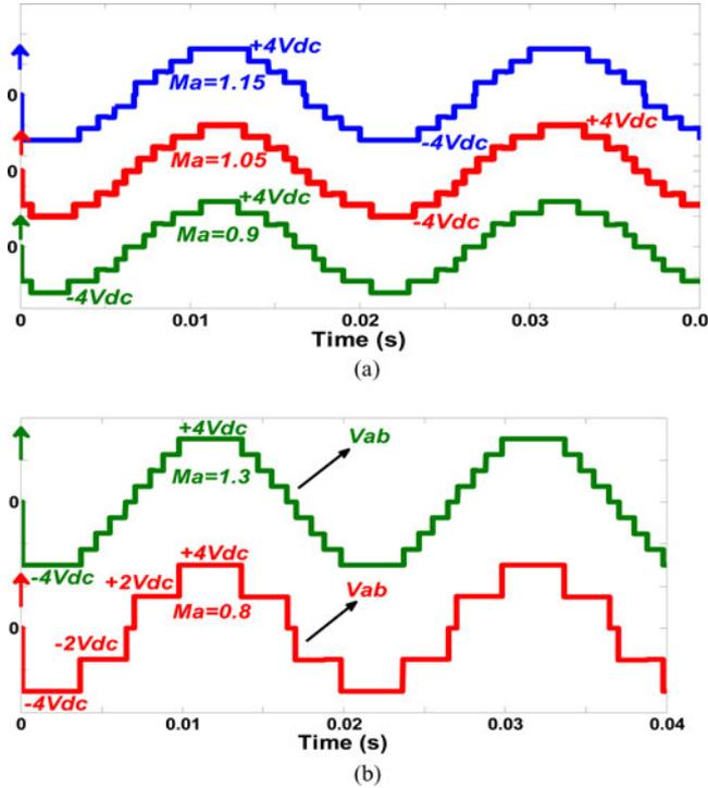
Fig. 6. Simulated waveforms of  $V_{ab}$  at different modulation indices for the proposed inverter: (a)  $M_a = 0.9, 1.05,$  and  $1.15$  and (b)  $M_a = 0.8$  and  $1.3$ .
