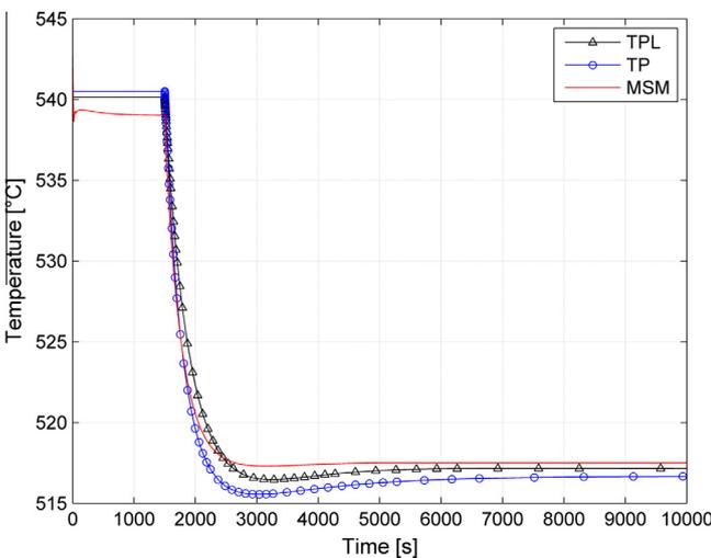
Fig. 6. Steam temperature at the superheater outlet section.
