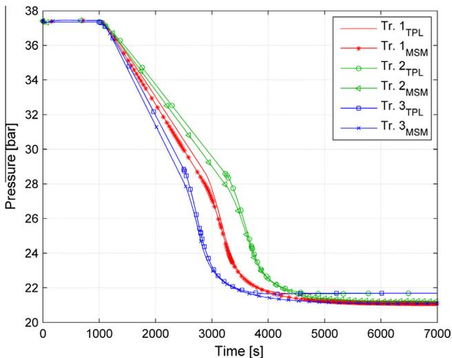
Fig. 13. Steam pressure into the drum during transients Tr. 1, Tr. 2 and Tr. 3.
