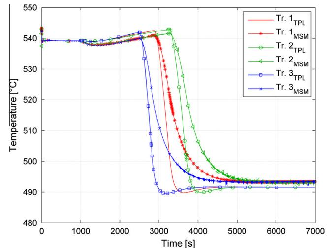
Fig. 12. Steam temperature at the superheater exit during transients Tr. 1, Tr. 2 and Tr. 3.
