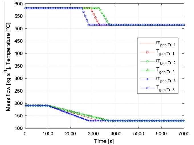
Fig. 10. Mass flow rate and temperature of exhaust gases at the HRSG inlet during transients Tr. 1, Tr. 2 and Tr. 3.
