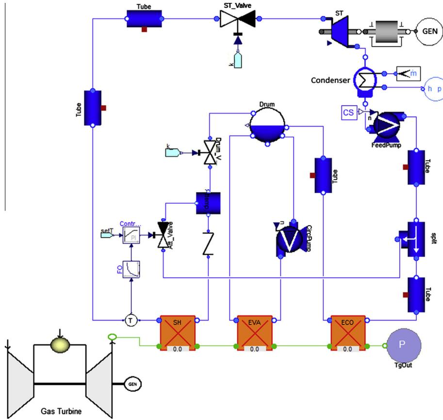
Fig. 1. Modelica object diagram of the single pressure Heat Recovery Steam Generator.
