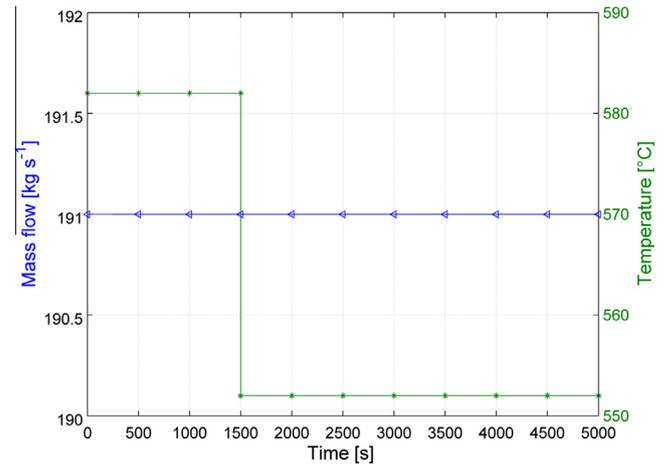
Fig. 4. Mass flow rate and temperature of the exhaust gasses at the HRSG inlet section.
