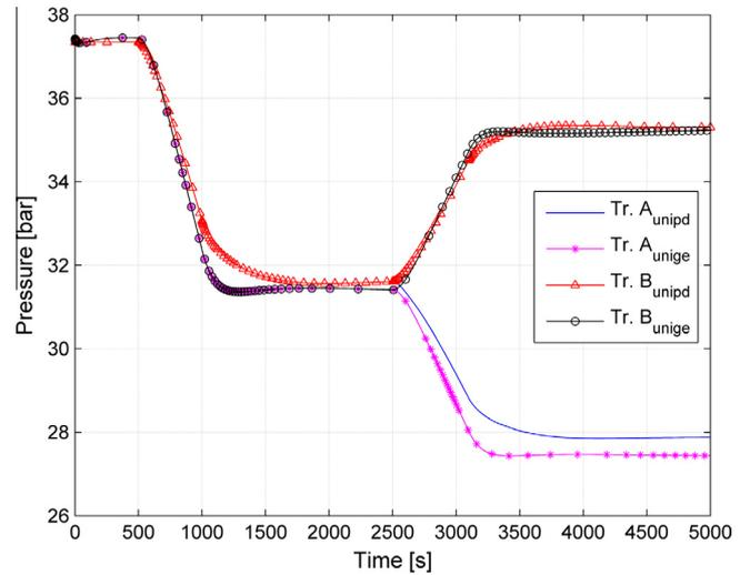
Fig. 8. The steam drum pressure during transients “Tr. A” and “Tr. B”.
