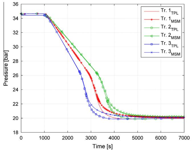
Fig. 11. Steam pressure at the superheater exit during transients Tr. 1, Tr. 2 and Tr. 3.
