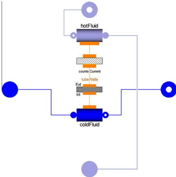
Fig. 3. Modelica object diagram of the heat exchanger model.
