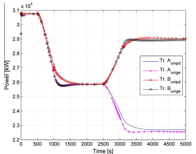
Fig. 9. Electric power produced by the electric generator during transients “Tr. A” and “Tr. B”.
