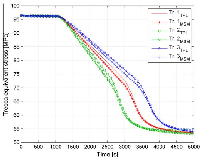
Fig. 14. The signed Tresca equivalent stress during transients Tr. 1, Tr. 2 and Tr. 3.
