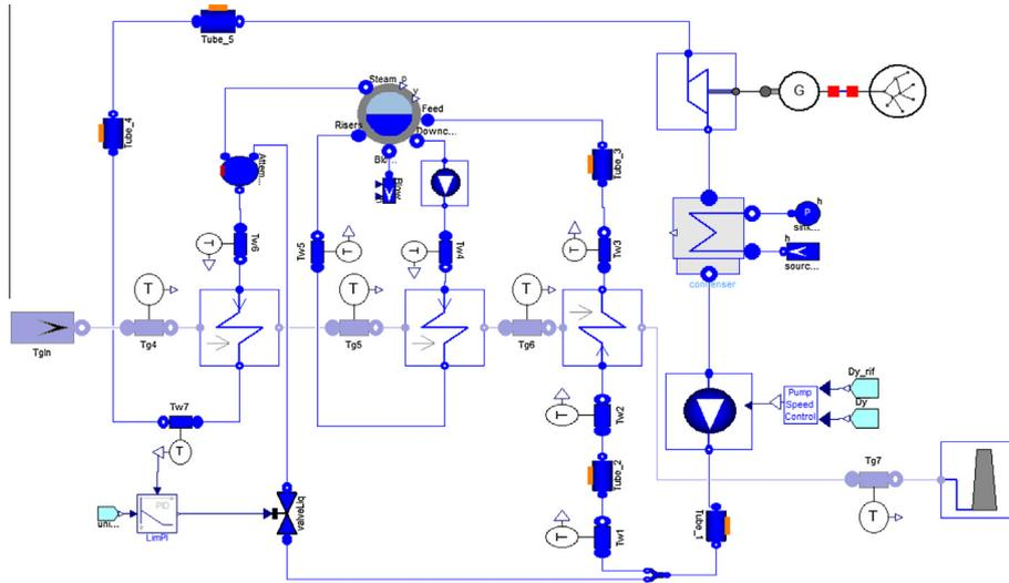
Fig. 2. Modelica object diagram of the single pressure Heat Recovery Steam Generator.
