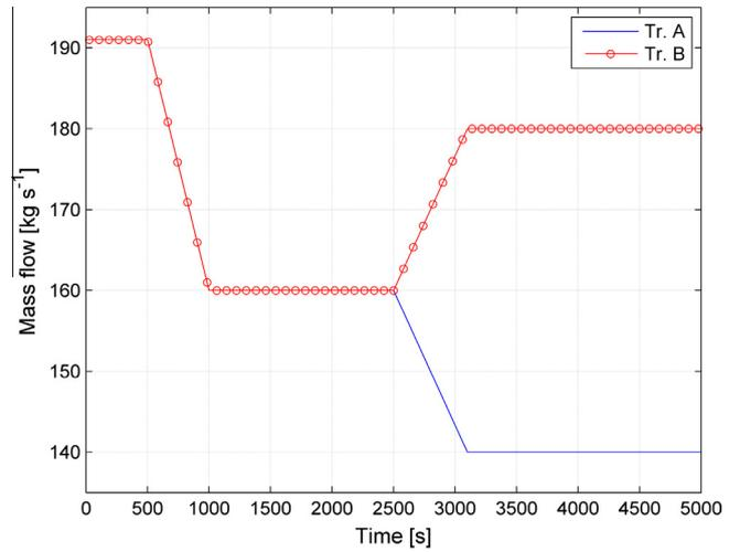
Fig. 7. The exhaust gas mass flow rate at the HRSG inlet for transients “Tr. A” and “Tr. B”.
