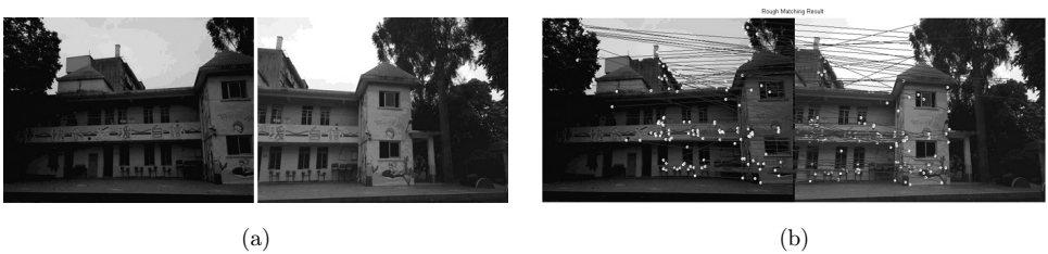
Fig. 10. First experiment: image stitching for the third set of images. (a) Images 2 and 4, (b) SIFT matches, (c) RANSAC inliers, (d) rendered with weighted average blending.
