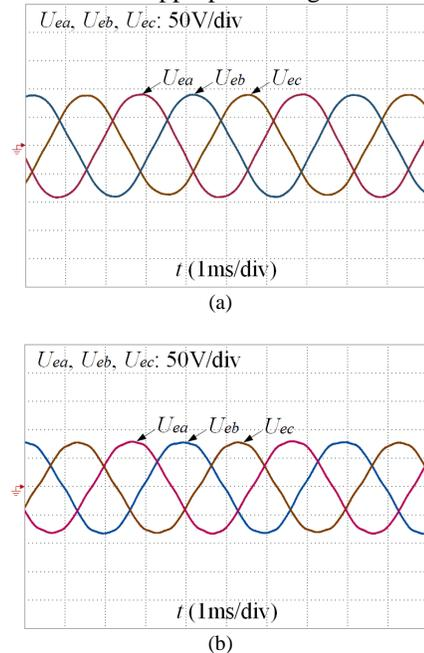
Fig. 14. Back EMF waveforms. (a) Regular PM length. (b) Short PM length.
