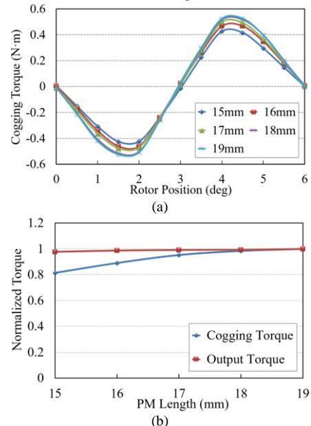
Fig. 7. Cogging torque and average output torque for inner-inner topology at different PM lengths. (a) Cogging torque. (b) Normalized average output torque and peak cogging torque.
