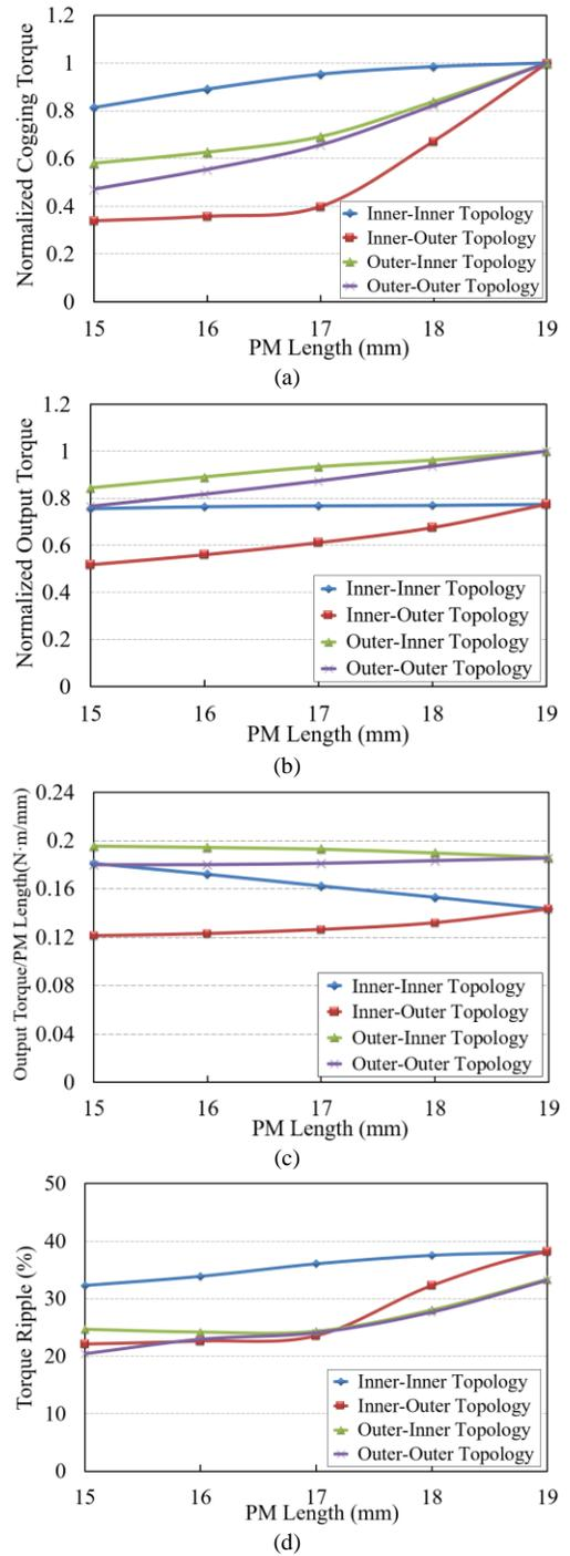
Fig. 11. Comparison of FSPM Machine Topologies. (a) Cogging torque. (b) Average output torque. (c) PM utilization ratio. (d) Torque ripple.
