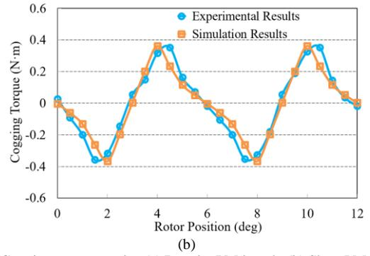
Fig. 13. Cogging torque results. (a) Regular PM length. (b) Short PM length.
