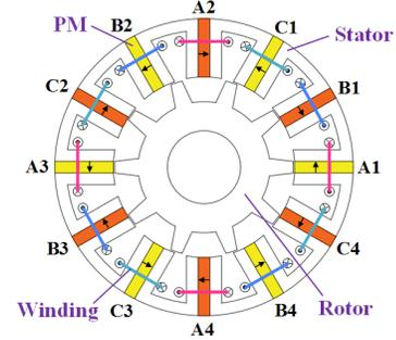
Fig. 1. Cross section of traditional FSPM machine.
