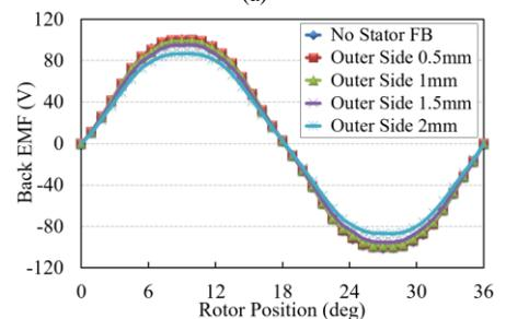
Fig. 3. Back EMF under different FB positions and thicknesses. (a) Inner side. (b) Outer side.
