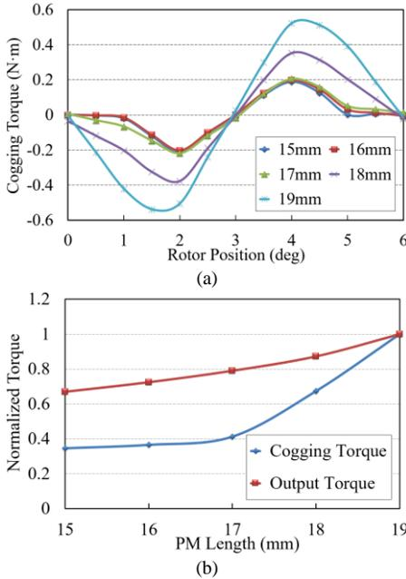
Fig. 8. Cogging torque and average output torque for inner-outer topology at different PM lengths. (a) Cogging torque. (b) Normalized average output torque and peak cogging torque.
