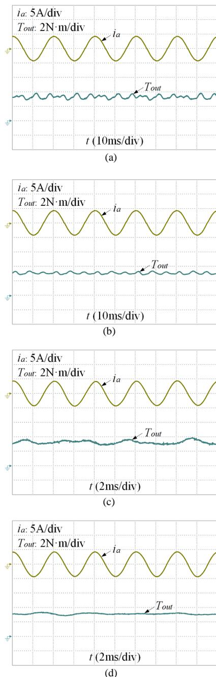
Fig. 15. Current and output torque waveforms. (a) Regular PM length topology at 300 r/min. (b) Short PM length topology at 300 r/min. (c) Regular PM length topology at 1500 r/min. (d) Short PM length topology at 1500 r/min.
