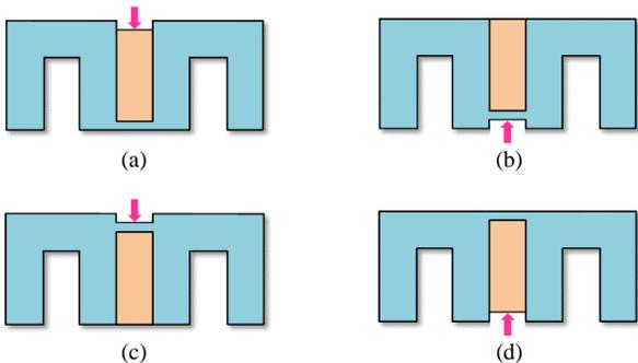
Fig. 5. Four FSPM machine topologies with short PM and stator FB. (a) Inner-inner topology. (b) Inner-outer topology. (c) Outer-inner topology. (d) Outer-outer topology.
