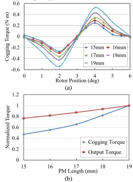
Fig. 10. Cogging torque and average output torque for outer-outer topology at different PM lengths. (a) Cogging torque. (b) Normalized average output torque and peak cogging torque.
