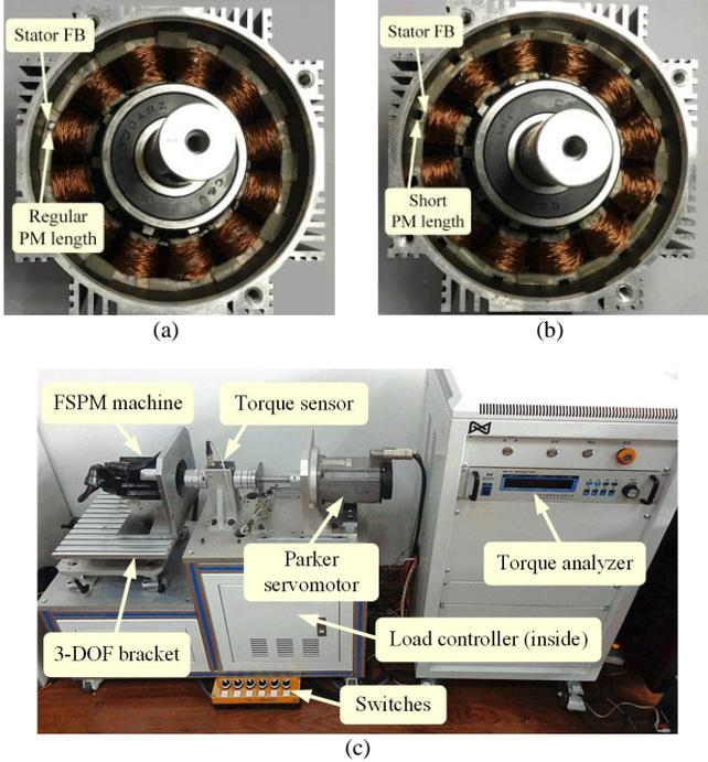
Fig. 12. Photographs of FSPM machines and experimental test-rig. (a) Outer-inner topology with regular PM length and FB. (b) Outer-inner topology with short PM length and FB. (c) Experimental test-rig.
