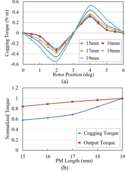
Fig. 9. Cogging torque and average output torque for inner-inner topology at different PM lengths. (a) Cogging torque. (b) Normalized average output torque and peak cogging torque.
