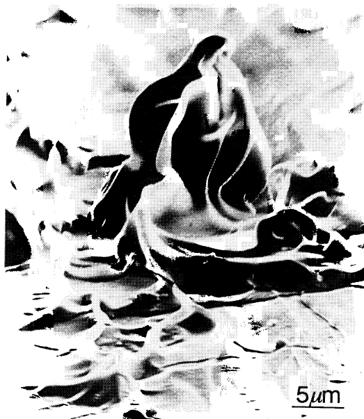
Fig. 11 Tensile fracture surface appearance of an amorphous Zr_{60}Al_{10}Co_3Ni_9Cu_{18} cylinder.
