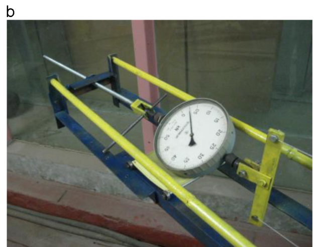
Fig. 14. Forces and displacements measurement. First series – horizontal location. (a) Forces. (b) Displacement.
