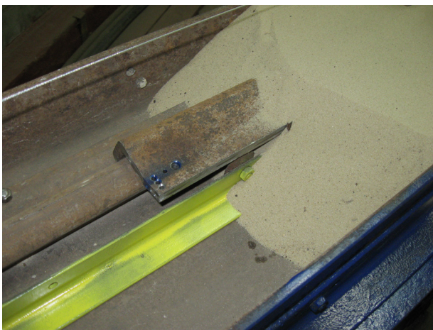
Fig. 13. Laboratory modeling of pile-pile friction with sandy soil in interlocks (first series – horizontal location). (a) Forces. (b) Displacement.
