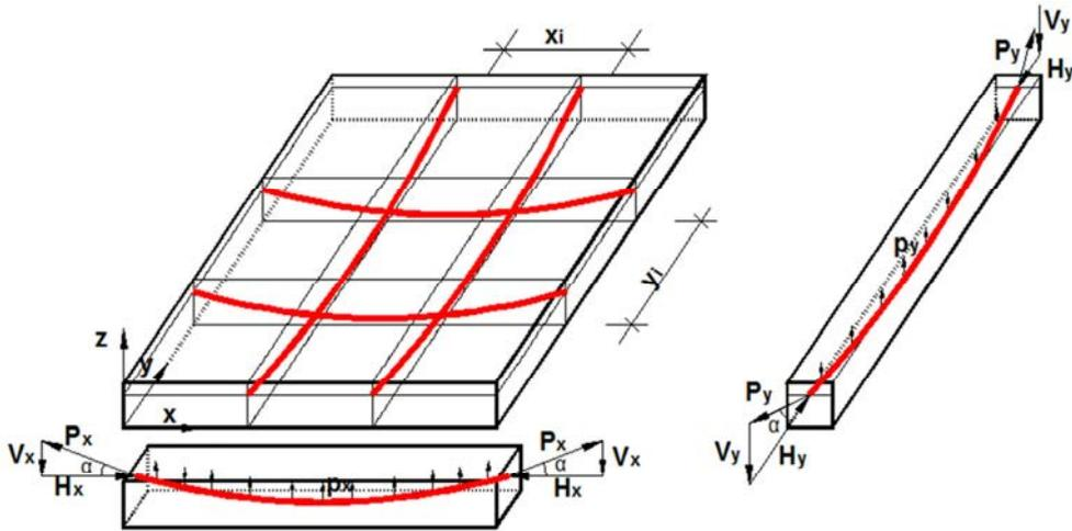
Fig. 4. Simply supported prestressed beam
