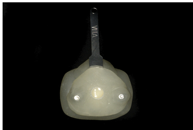
2 Acrylic resin device with cover allowing only consistent thirds of the shade tab to be measured.
