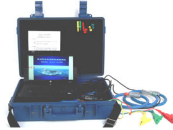
Fig. 7. Motor incipient failure online detector.
