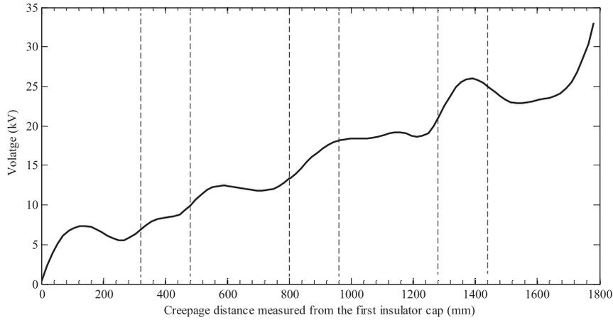
Fig. 5. Voltage distribution along creepage distance.
