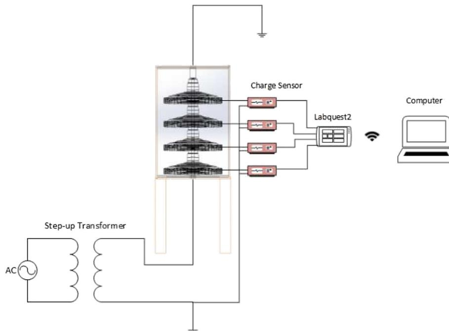
Fig. 11. Charge measurement experimental setup.
