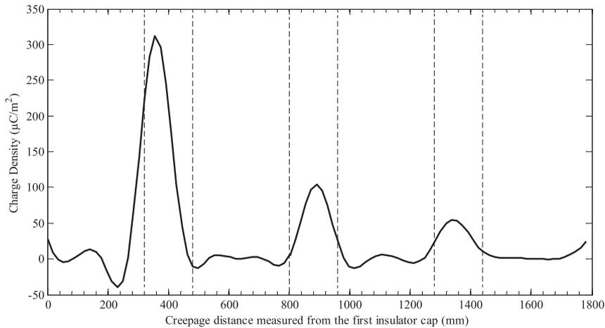
Fig. 7. Charge density distribution along creepage distance.
