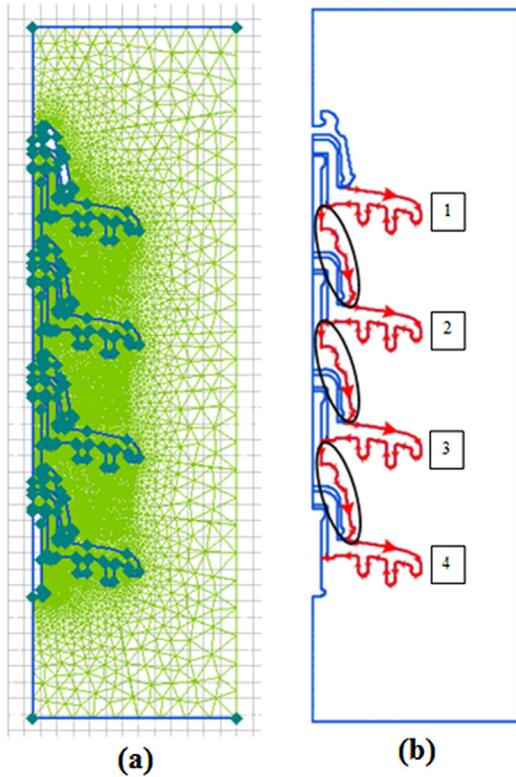
Fig. 3. (a) Mesh model, and (b) creepage distance (red in colour). (For interpretation of references to colour in this figure legend, the reader is referred to the web version of the article.)
