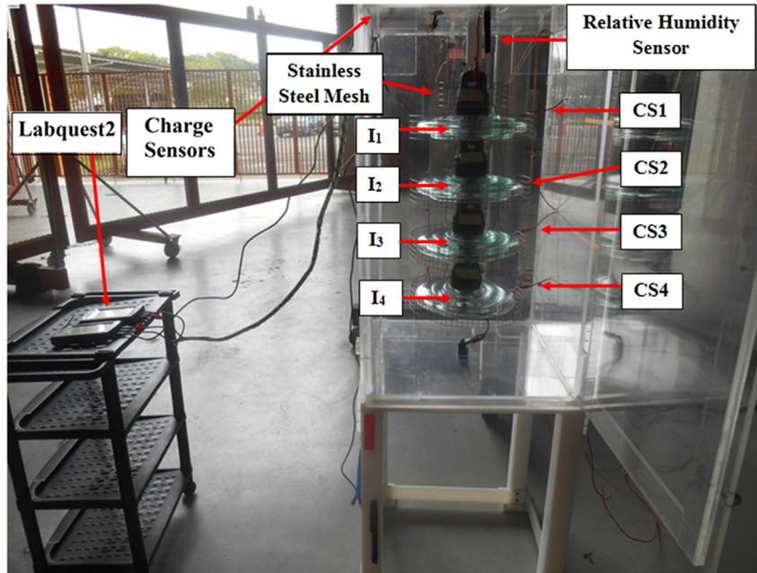
Fig. 10. Pictorial view of the laboratory test setup.
