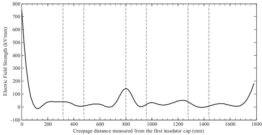
Fig. 6. Electric field distribution along creepage distance.
