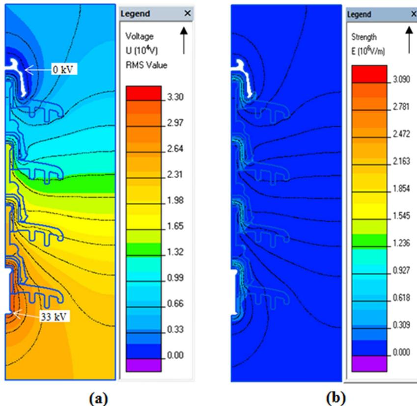
Fig. 4. (a) Voltage distribution, and (b) electric field distribution.
