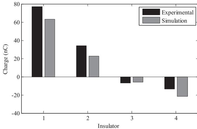
Fig. 12. Charge distribution on each insulator.
