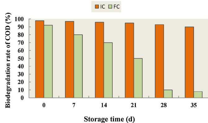
**Fig. 8.** Storage stability of COD biodegradation activity by immobilized cells of activated sludge in PVA-GA beads.
