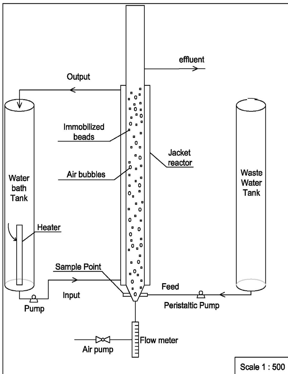
**Fig. 2.** Schematic diagram of the lab-scale pilot plant.
