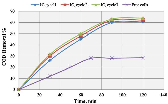
**Fig. 3.** Efficiency of COD removal from real-field petroleum wastewater in SBBR using non-adopted immobilized mixed cells and free cells.
