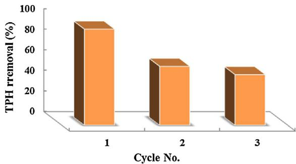
**Fig. 4.** TPH reduction (%) as a function of cycle of immobilized cells of activated sludge in PVA-GA beads reuse.
