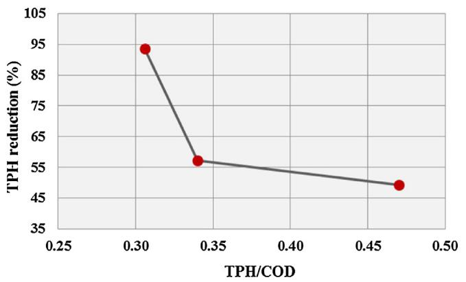
**Fig. 5.** TPH reduction (%) as a function of (TPH/COD) ratio.
