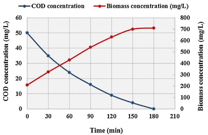
**Fig. 6.** Biomass growth versus COD degradation in PVA-GA beads.
