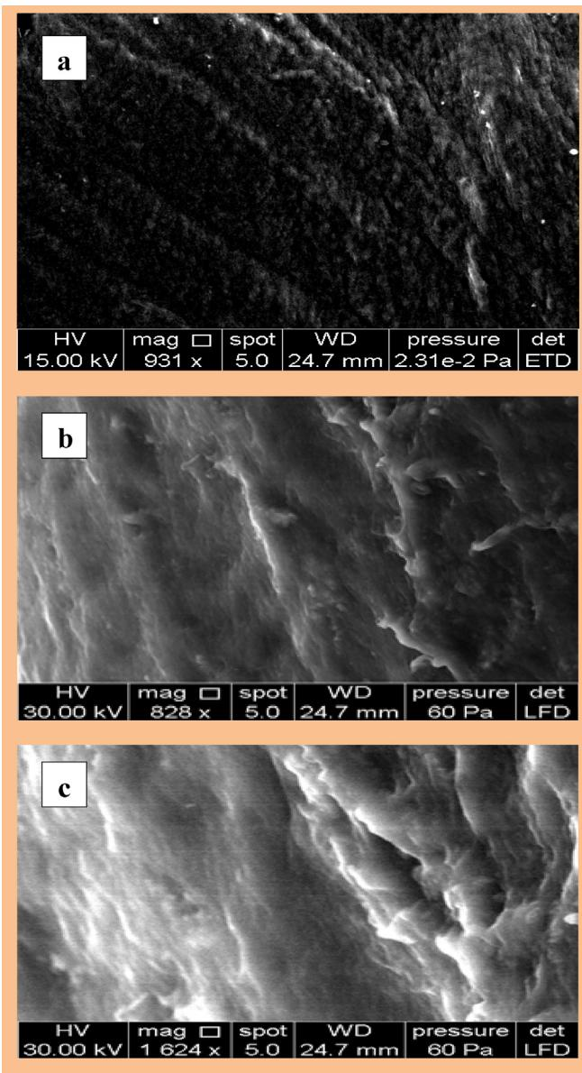
**Fig. 7.** SEM for the beads; (a) blank beads, (b) beads with cells before biodegradation, and (c) beads with cells after biodegradation.
