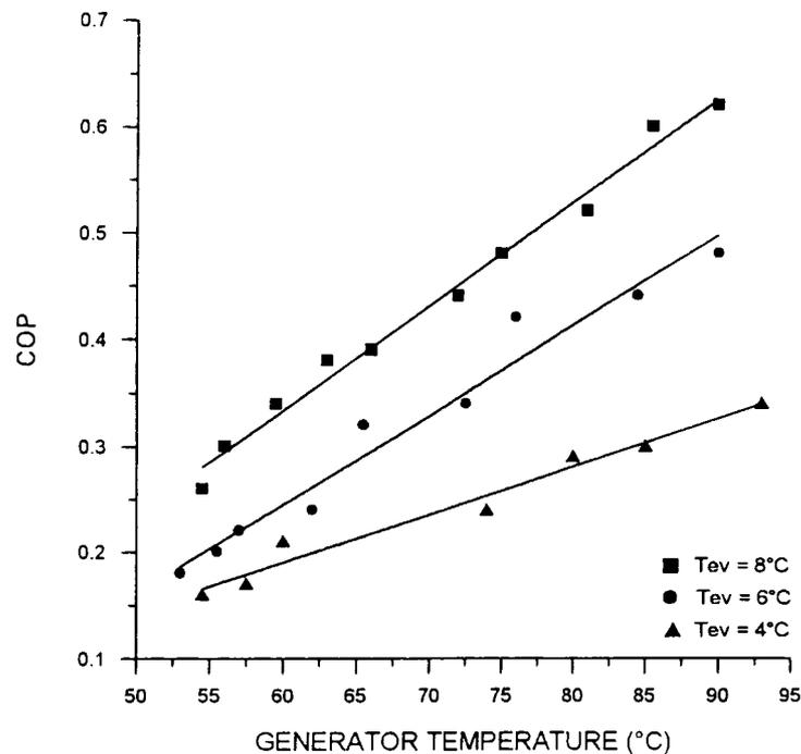
Fig. 4. The change in the COP with the generator temperature at the various evaporator temperatures.
