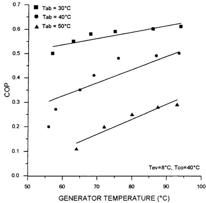
Fig. 7. The change in the COP with the generator temperature at the various absorber temperatures.
