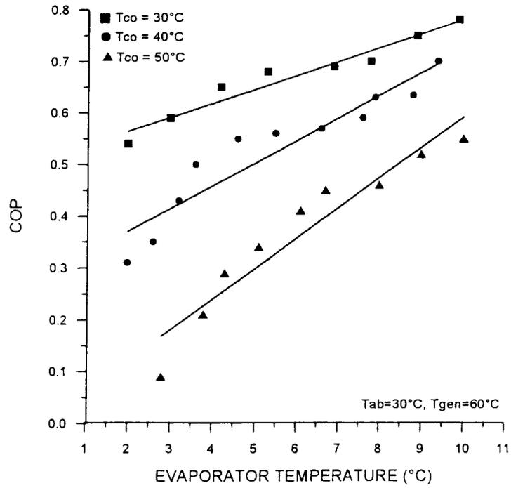
Fig. 5. The change in the COP with the evaporator temperature at the various condenser temperatures.
