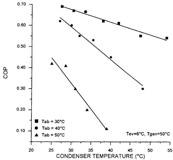
Fig. 8. The change in the COP with the condenser temperature at the various absorber temperatures.
