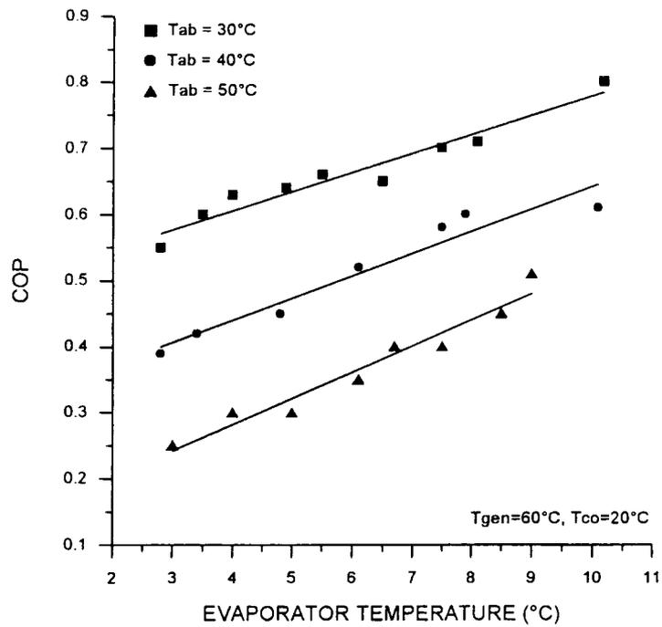
Fig. 6. The change in the COP with the evaporator temperature at the various absorber temperatures.
