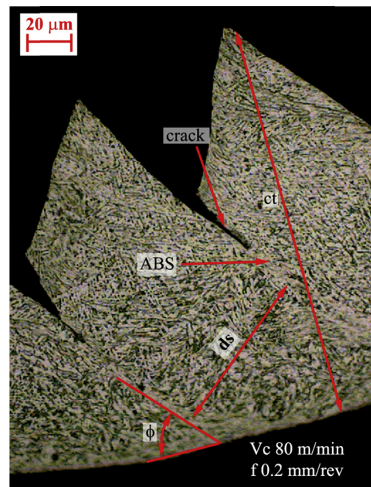
Fig. 10. Cross-section of the chip generated under cryogenic cooling with indication of the measured chip features.
