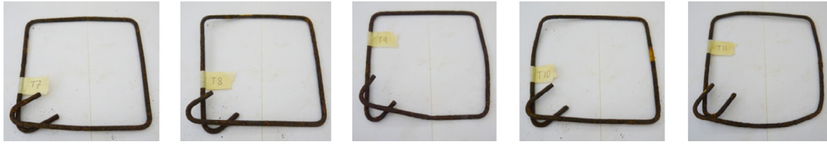
Fig. 11. Appearance of some typical corroded transverse reinforcing bars of specimen AS1 ( X_{corr} = 9.5\% ) after testing and removing all the rust.
