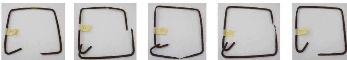
Fig. 13. Appearance of some typical corroded transverse reinforcing bars of specimen AS3 ( X_{corr} = 25.0\% ) after testing and removing all the rust.
