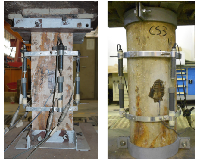
Fig. 3. Typical test set-up of square and circular specimens in 5000 kN capacity hydraulic universal testing machine.
