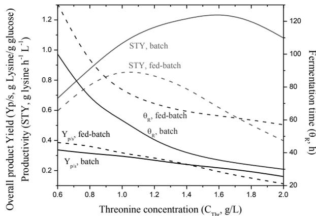
Figure 2. Overall product yield, productivity and reaction time for batch and fed-batch operations.
