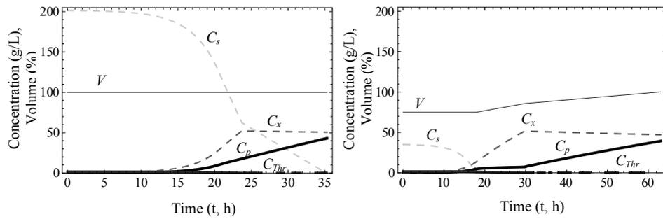
Figure 1. Dynamic behaviour of the fermentation reactor to produce L-lysine: (a) batch operation and (b) fed-batch operation, under similar conditions ( $c_{Thr,0} = 1.6$  g/L).
