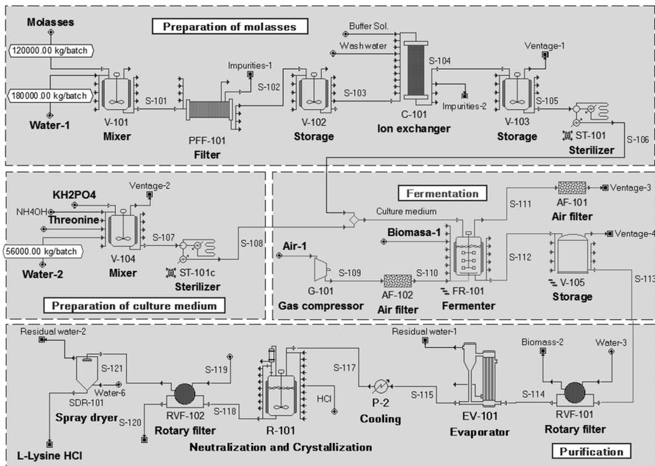
Figure 3. Flowsheet for the production process of L-lysine .
