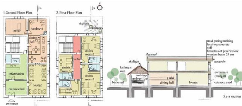
Fig. 2 Proposal, (a) ground floor, (b) first floor, (c) section
