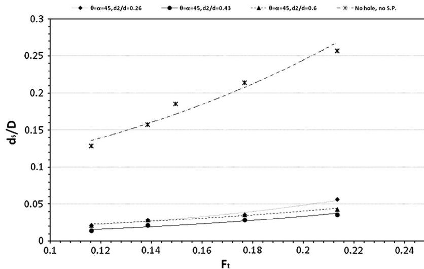
Figure 8 Relation between the relative scour depth  $d_s/D$  and Froude number  $F_t$  for different relative perforation diameters of the S.P.
