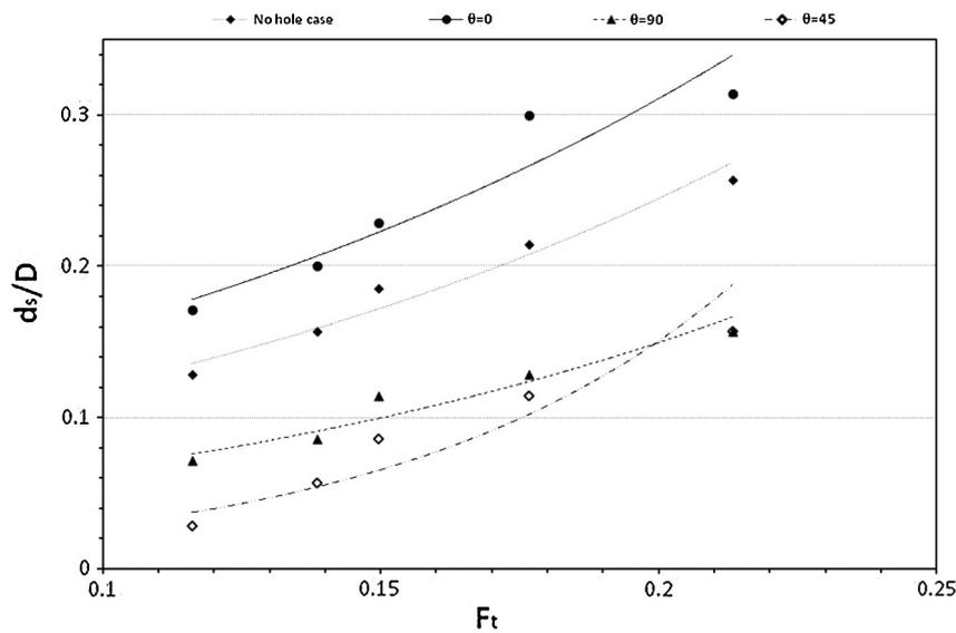
Figure 5 Relation between the relative scour depth  $d_s/D$  and Froude number  $F_t$  for different hole angles of the perforated pile.
