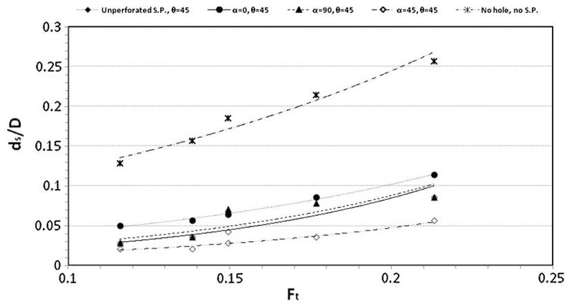
Figure 7 Relation between the relative scour depth  $d_s/D$  and Froude number  $F_t$  for using a perforated S.P.
