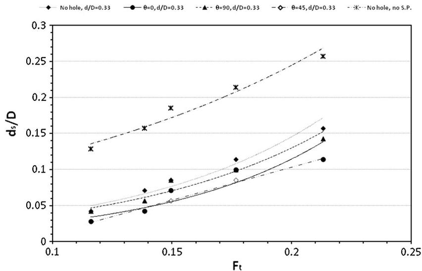
Figure 6 Relation between the relative scour depth  $d_s/D$  and Froude number  $F_t$  for using combined countermeasures.
