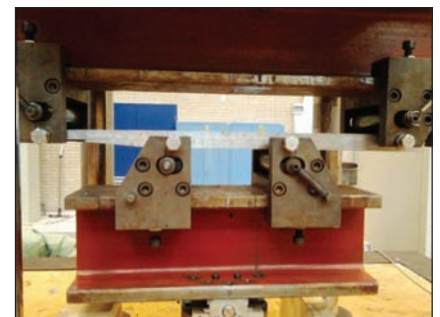
Fig. 11: Test set-up to determine S-N curve
