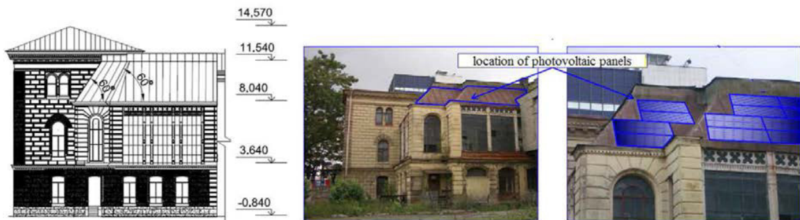
Fig. 10. The initial project solution assumed photovoltaic panels placed on the southward roof of the greenhouse building
