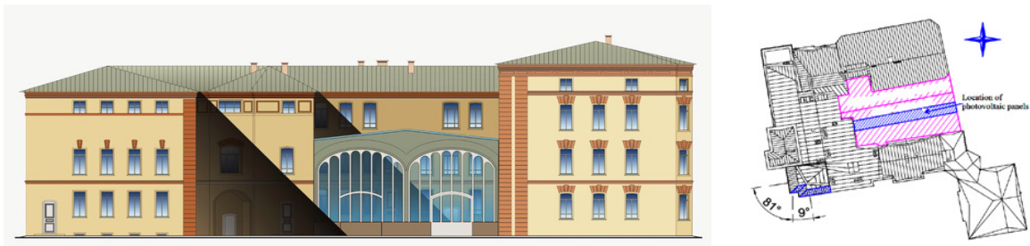
Fig. 11. Model of the inner yard made of the glass. Photovoltaic panels to be placed on the southward slope of the yard glass coverage.
