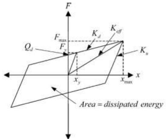
Fig. 2. Characteristic of LRB system
