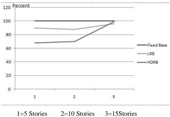
Fig. 11: Deducted Percent for the weight of structure in compare with fixed base as the index (100%)
