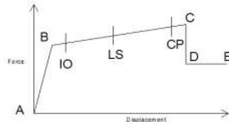
Fig. 4. FEMA Force-Displacement relation
