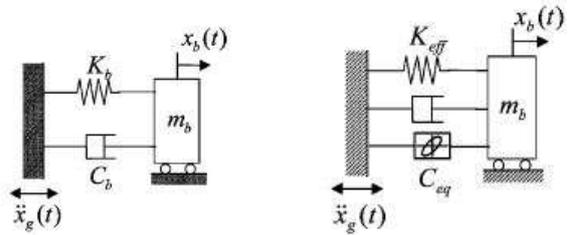
Fig 1. RB/HDRB model LRB model
