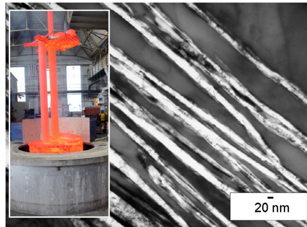
Figure 3. Extremely thin plates of bainitic ferrite embedded in a matrix of austenite. Inset: large-scale processing of new steel.
