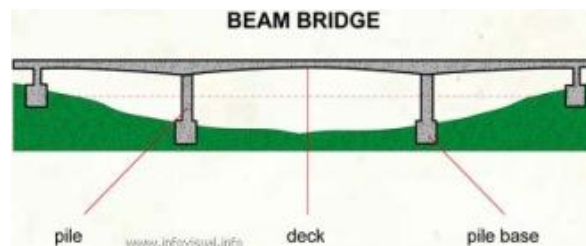
Figure 1. The structure of Beam Bridge
