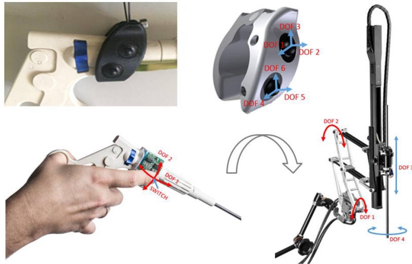
Fig. 2. Prototype mini-joystick integrated in a laparoscope (top left) to control robotic arm movement.
