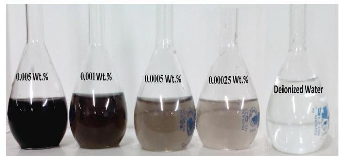
Fig. 1. Samples of the nanofluids by different weight percent.
