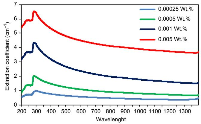
Fig. 7. Extinction coefficient values of samples in different wavelengths.
