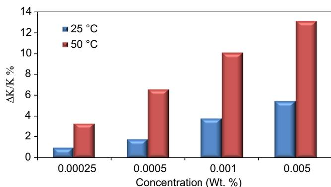
**Fig. 10.** thermal conductivity ratios of nanofluids with different wt% at 25 and 50 °C. increase effective surface of thermal conductivity, in this part we investigate the importance of increase in nanofluids weight percent compared to increase in temperature than thermal conductivity coefficient. Results from experimental measurement are shown in Fig. 9.
