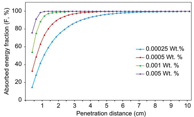
Fig. 8. Absorbed energy fractions ( $F$ ) versus the penetration distance ( $X$ ) for the nanofluids at different wt%.
