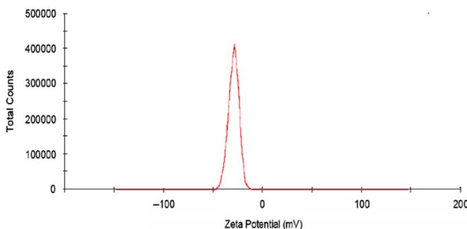
Fig. 4. Zeta potential value of nanofluid with weight percent of 0.005.
