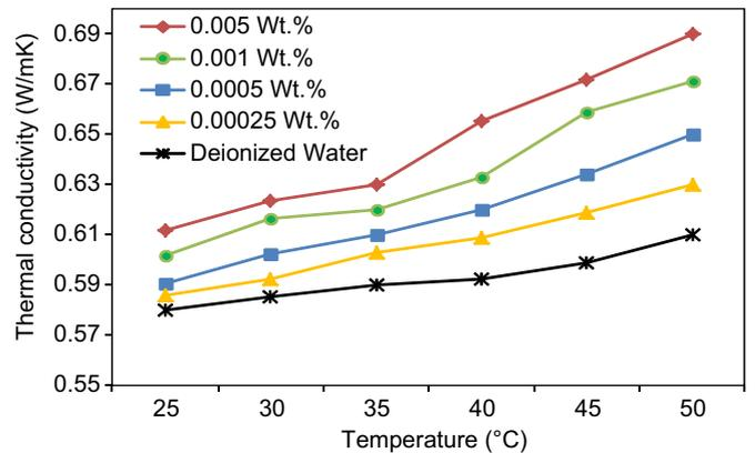
Fig. 9. Thermal conductivity of nanofluid samples and deionized water at different temperatures.
