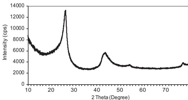
Fig. 3. The results of X-ray diffraction graphene nanoplatelets.
