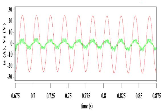
Figure 3. Input current and voltage ( $V_s/2$ ) during steady state operation with reactive power minimization
