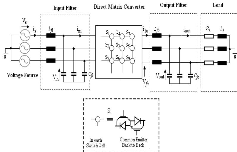
Figure 1. Direct Matrix Converter power supply topology
