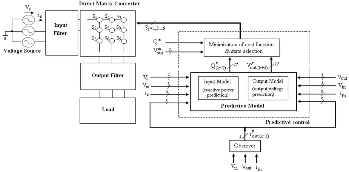
Figure 2. Control scheme of Model Predictive Control
