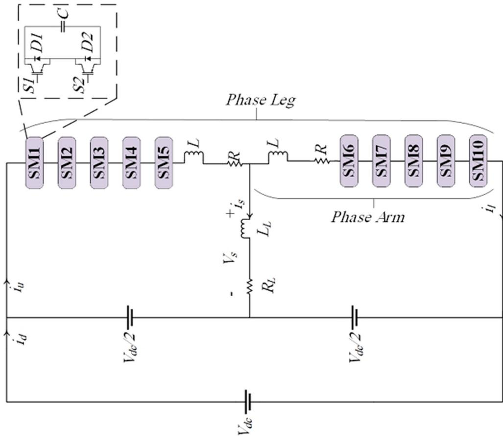
Fig. 1. Topology of a single-phase MMC with 10 SMs
