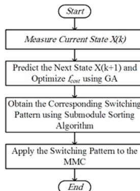
Fig. 2. The proposed control algorithm
