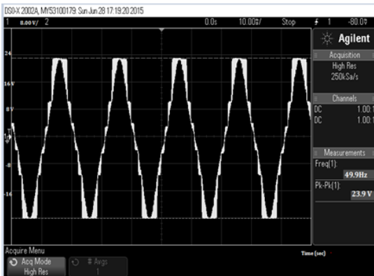
Fig 10. Hardware output result of Z-source multilevel inverter.
